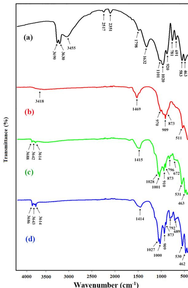
Fig. 2 FT-IR spectra of (a) standard ceramic tile, (b) electric arc furnace (EAF) steel slag, (c) ceramic tile including 10.0 wt% EAF, and (d) ceramic tile including 40.0 wt% EAF.
