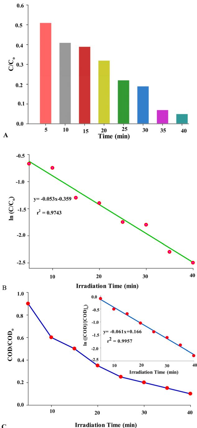
Fig. 7 (A) and (B) CEF photodegradation results versus time, and (C) COD results of the solutions obtained in case A (inset: the corresponding Hinshelwood plot).
