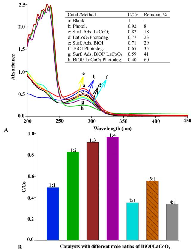
Fig. 5 (A) UV-Vis CEF absorption spectra over the applied removal processes (0.3 g L<sup>-1</sup> of each catalyst in 10 mL of 10 mg L<sup>-1</sup> CEF solution, time: 40 min, the mole ratio of BiOI : LaCoO<sub>3</sub> was 1 : 1); (B) the effect of the variation in the BiOI:LaCoO<sub>3</sub> molar ratio of the coupled catalyst on the CEF photodegradation.
