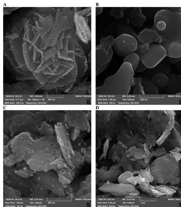
Fig. 3 SEM images of BiOI (A), LaCoO<sub>3</sub> (B) and LaCoO<sub>3</sub> (4.0 wt%)/BiOI hybrid (C) and (D).
