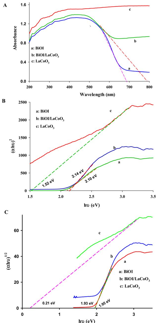
Fig. 2 (A) UV-Vis DRS absorption spectra of BiOI, LaCoO<sub>3</sub>, and LaCoO<sub>3</sub>/BiOI samples. (B) and (C) Tauc plots for  $E_g$  estimation for  $n = 2$  and  $n = 1/2$ .
