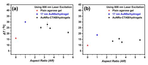
Fig. 5 Temperature changes measured after 15 minute heating under 808 nm laser exposure for plain agarose (red triangles), Au NSs/hydrogel (17 nm, blue circles), and Au NR/hydrogels with varying aspect ratios (black squares) at (a) 5 mm and (b) 15 mm distance from the heating spot (N = 3). The data illustrate the impact of the particle size and shape on heat transfer and thermal responses. Symbols represent mean values, and vertical bars indicate standard deviations
