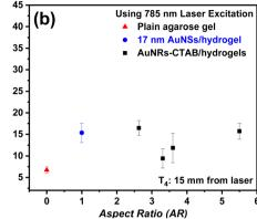
Fig. 4 Temperature changes measured after 15 minute heating under 785 nm laser exposure for plain agarose (red triangles), Au NSs/hydrogel (17 nm, blue circles), and Au NR/hydrogels with varying aspect ratios (black squares) at (a) 5 mm and (b) 15 mm distance from the heating spot (N = 3). The data illustrate the impact of particle shape and size on heat transfer and thermal responses. Symbols represent mean values, and vertical bars indicate standard deviations
