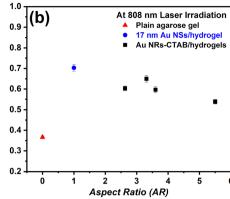
Fig. 8 Photothermal conversion efficiencies as a function of AR using (a) 785 nm and (b) 808 nm laser excitation wavelength. Symbols represent the mean value, and vertical bars indicate the standard deviation
