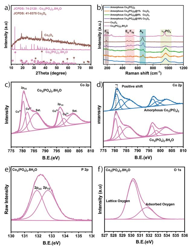
Fig. 1 (a) XRD pattern, (b) Raman, (c) XPS Co 2p, (d) XPS comparison of the prepared crystalline  $Co_3(PO_4)_2 \cdot 8H_2O$  and amorphous  $Co_3(PO_4)_2 \cdot (e)$  XPS P 2p and (f) XPS O 1s.
