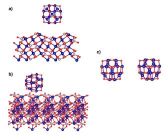
Fig. 5 (a) Side and (b) inclined views of the optimized structure of adsorbed  $\text{Co}_3\text{O}_4$  nanoparticles on the  $\text{Co}_3(\text{PO}_4)_2$  surface. (c) Optimized structure of the two  $\text{Co}_3\text{O}_4$  nanoparticles. Co, P and O atoms are represented by blue, purple and red balls, respectively.
