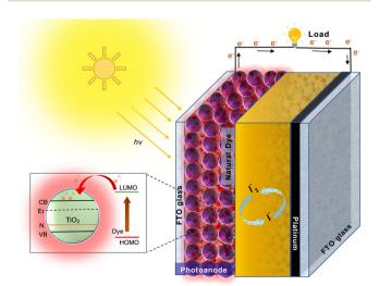
Fig. 1 Basic components and mechanism of DSSCs.
