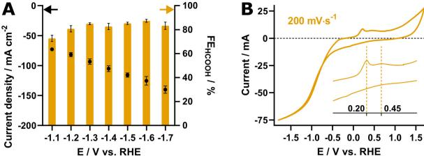
Fig. 2 (A) Current densities (black) and faradaic efficiencies (orange) resulting from the potential screening of the Pom. SnO<sub>2</sub>aC catalyst. All measurements were carried out in triplicate; (B) cyclic voltammogram of the SnO<sub>2</sub>@C catalyst recorded at 200 mV s<sup>-1</sup> under conditions identical to those during eCO<sub>2</sub>R.
