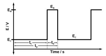
Fig. 1  $\,$  Example of an applied pulse profile for pulsed electrochemical  ${\rm CO_2}$  reduction.
