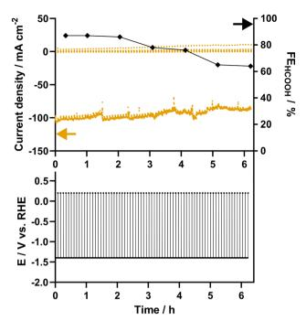
Fig. 5 Current density (orange) and faradaic efficiency (black) towards formate and pulse profile resulting from a p-eCO<sub>2</sub>R experiment with  $t_c$  = 300 s,  $E_c = -1.4$  V vs. RHE,  $t_a = 10$  s and  $E_a = 0.2$  V vs. RHE (p-0.20-10).
