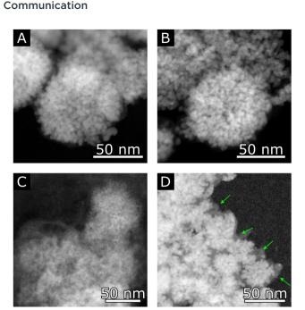
Fig. 7 HAADF-STEM images of the SnO2@C catalyst in (A) it's pristine form; (B) and (D) after 6 h of p-eCO<sub>2</sub>R under the p-0.20-30 regime; (C) after 6 h of p-eCO<sub>2</sub>R under the p-0.45-10 regime. In (D), the carbon shell, which remained intact after 6 h of p-0.20-30, is indicated with green arrows
