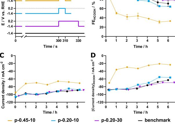
Fig. 6 (A) Pulse profiles, (B) faradaic efficiencies towards formate, (C) current densities and (D) partial current densities formate production for 6 h (p)-eCO<sub>2</sub>R experiments labelled p-0.45-10 (orange), p-0.20-10 (blue), p-0.20-30 (magenta) and the potentiostatic benchmark experiment (black).
