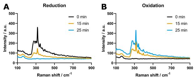
Fig. 3 Region of interest of the in situ Raman spectra of SnO<sub>2</sub>@C pomegranates under (A) reductive and (B) oxidative conditions. Both images show the spectra recorded at the start, after 15 and after 25 minutes, respectively.
