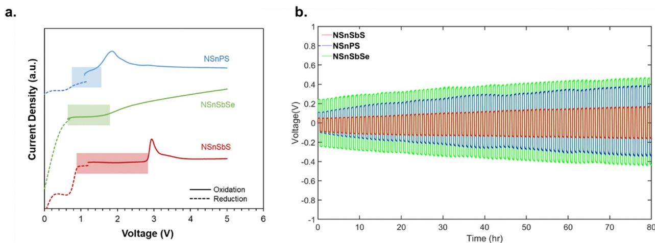
Fig. 7 (a) Linear sweep voltammetry of Na<sub>11</sub>Sn<sub>2</sub>PnCh<sub>12</sub> (Pn = P, Sb; Ch = S, Se) cells with a voltage range of 0–5 V at a scan rate of 0.1 mV s<sup>-1</sup>, and (b) cyclability of Na–Sn|Na<sub>11</sub>Sn<sub>2</sub>PCh<sub>12</sub>|Na–Sn symmetric cells at RT with a stacking pressure of 50 MPa.
