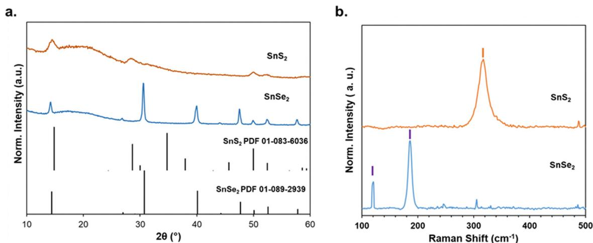
Fig. 1 (a) XRD and (b) Raman spectra of SnCh<sub>2</sub> (Ch = S, Se) recovered from metathesis reactions after annealing at 300 °C.
