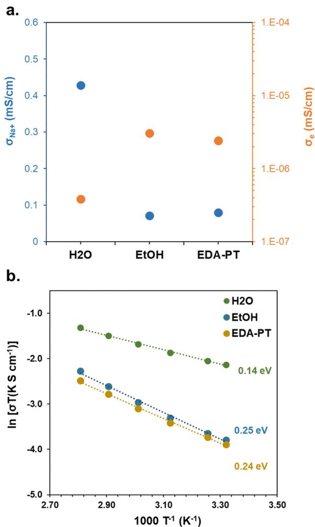
Fig. 5 (a) Ionic and electronic conductivity, and (b) Arrhenius plots of NSnSbS obtained from H<sub>2</sub>O, EtOH, and EDA-PT solvents, and further annealed at 550 °C.
