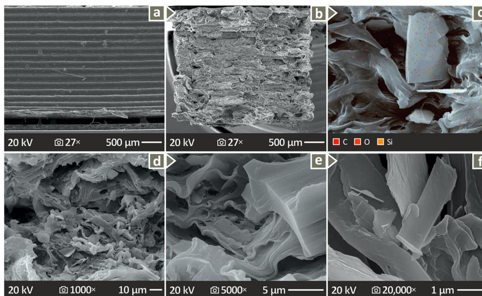
Fig. 12 SEM images of the PHA/1.5 wt% biochar: (a) lateral surface magnified at 27 $\times$ , (b) vertical surface magnified 27 $\times$ , (c) C, O, and Si elemental distribution through EDS, and (d)–(f) side surface magnified 1000 $\times$ , 5000 $\times$ , and 20 000 $\times$ .
