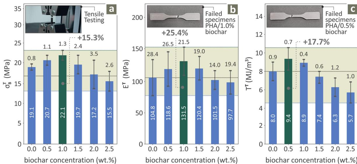
Fig. 7 Tensile results for the 3D-printed PHA/biochar (0.0, 0.5, 1.0, 1.5, 2.0, and 2.5 wt%) specimens: (a) tensile strength and an image from the tensile testing of a randomly selected specimen, (b) tensile modulus of elasticity and an image from a PHA/1.0 wt% biochar failed tensile specimen, and (c) tensile toughness, and an image from a PHA/0.5 wt% biochar failed tensile specimen.
