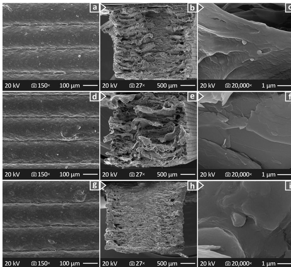
Fig. 11 SEM images showing (a)–(c) unfilled PHA, (d)–(f) PHA/1.0 wt% biochar and (g)–(i) PHA/2.0 wt% biochar: lateral surfaces at 150 $\times$  magnification, and fractured surfaces at 27 $\times$  and 20 000 $\times$ .
