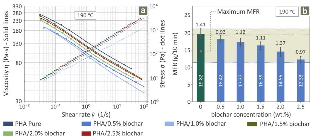
Fig. 4 Rheology results for PHA/biochar (0.0, 0.5, 1.0, 1.5, 2.0, and 2.5 wt%) composite samples (a) stress and viscosity versus shear rate results and (b) MFR levels.
