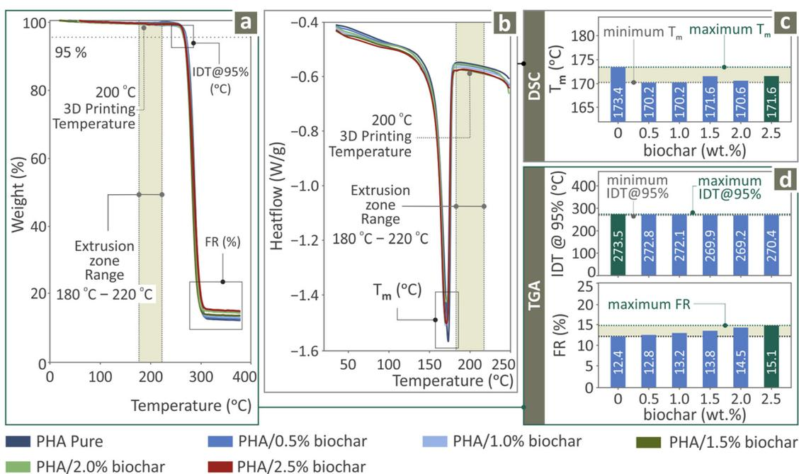
Fig. 5 Thermal property results of pure PHA and PHA/biochar (0.0, 0.5, 1.0, 1.5, 2.0, and 2.5 wt%) composite samples through (a) TGA and (b) DSC curves, as well as the respective measured (c)  $T_m$ , (d) FR, and IDT values.
