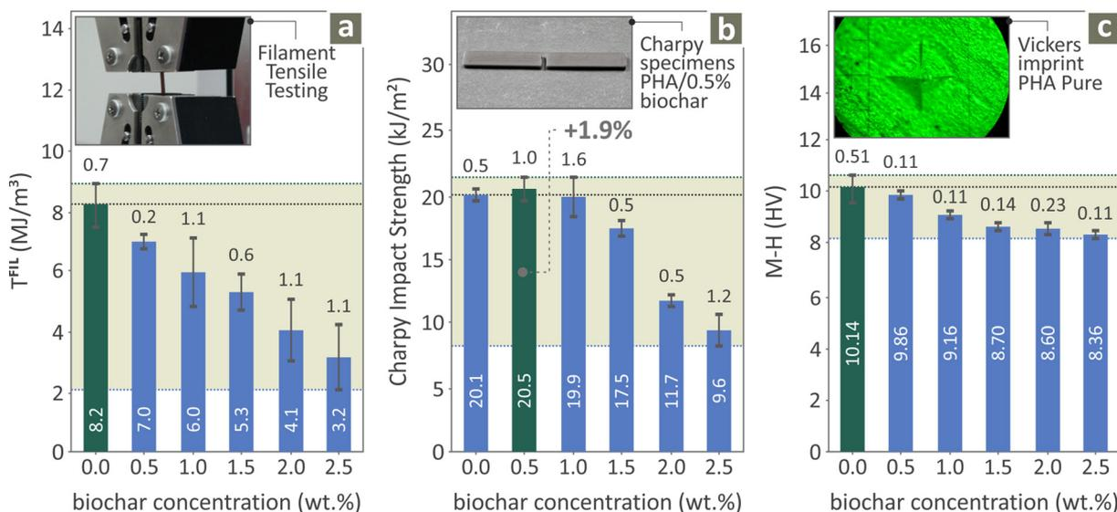
Fig. 9 Mechanical characterization results of PHA/biochar samples for all filler concentrations, to derive: (a) tensile toughness of the extruded filaments, (b) Charpy impact strength of the 3D-printed specimens, and (c) microhardness.
