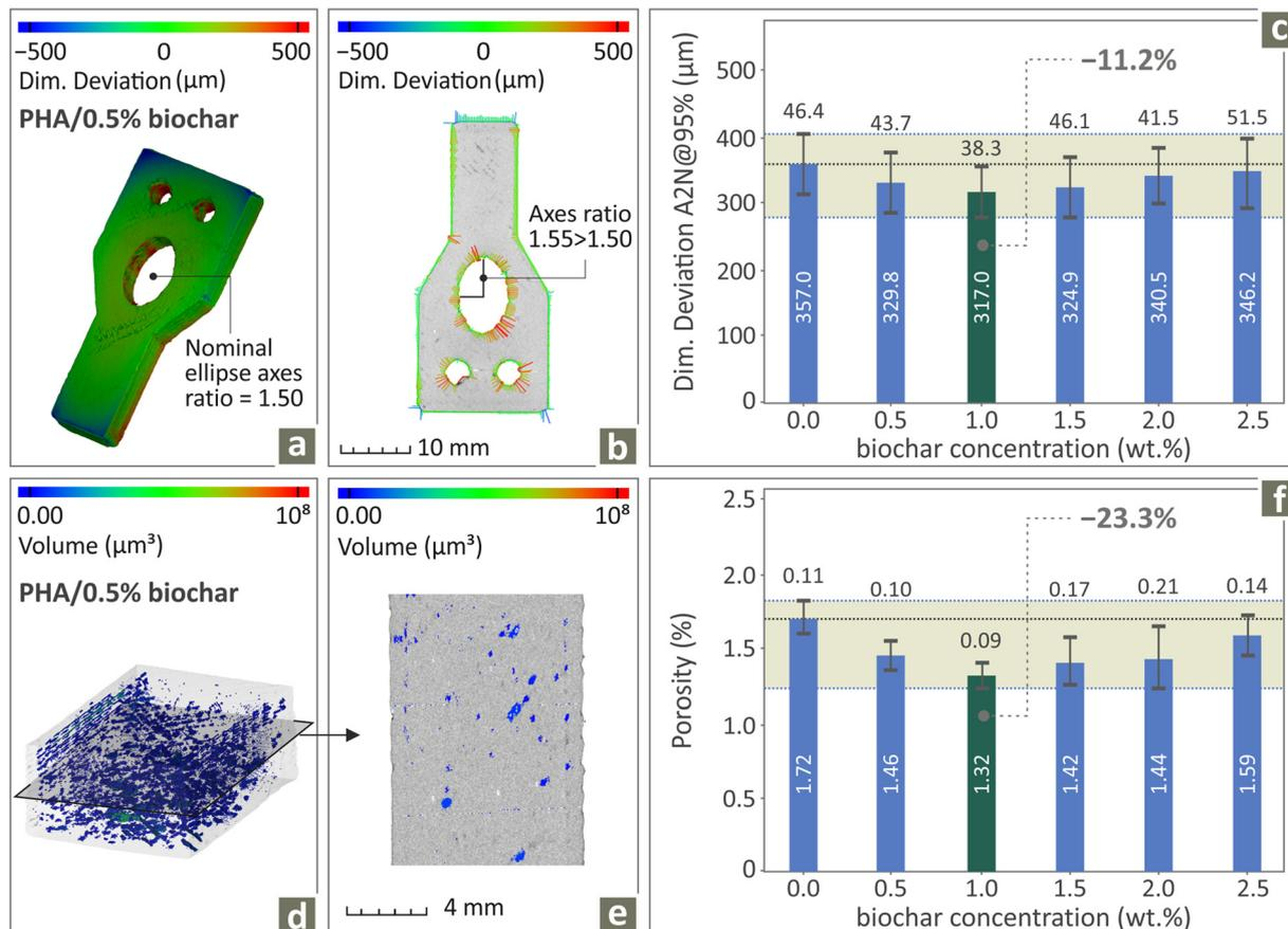
Fig. 10 (a) and (b) Dimensional deviation of a PHA/0.5 wt% biochar example through color-coded mapping, (c) geometrical accuracy values of all PHA/biochar samples, (d), (e) PHA/0.5 wt% biochar section through color-coded mapping, and (f) porosity values of all PHA/biochar samples.
