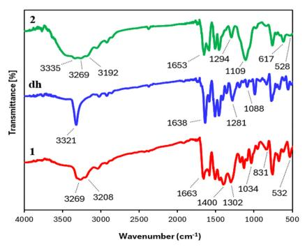
Fig. 1 Comparative vibrational spectra of complex 1 (red), complex 2 (green), and parent ligand dh (blue).
