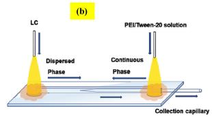
Fig. 1 (a) Photograph of the flow-focusing microfluidic device. (b) Schematic diagram illustrating the direction of fluid flow within the microfluidic device.
