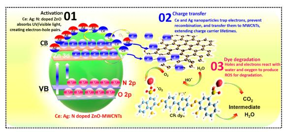
Fig. 13 Proposed photocatalytic mechanism of dye degradation using Ce/Aq/N-doped ZnO-MWCNT nanocomposites, demonstrating charge transfer pathways, reactive oxygen species formation, and pollutant degradation under visible light.
