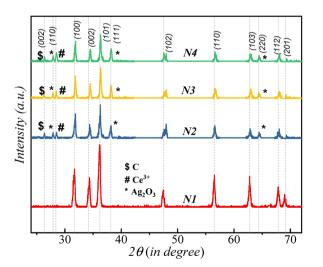
Fig. 2 XRD patterns of Ce/Ag/N-doped ZnO-MWCNT nanocomposites with varying Ce concentrations, confirming phase purity, crystallinity, and the presence of dopants.
