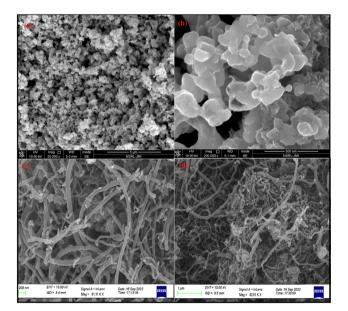
Fig. 5 FESEM images of (a) and (b) undoped ZnO (N1) and (c) and (d) Ce/ Ag/N-doped ZnO-MWCNT nanocomposites (N4), showing morphological transformations, and the formation of nanorod-like structures.
