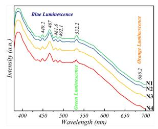
**Fig. 8** Photoluminescence spectrum of different nanocomposites, demonstrating reduced emission intensity in doped samples due to suppressed electron–hole recombination, which enhances photocatalytic efficiency.
