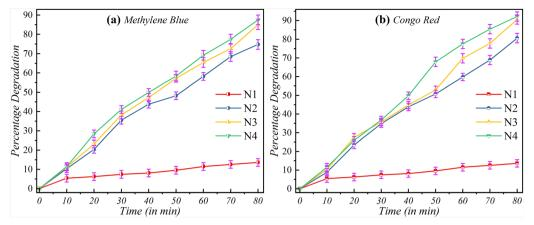
Fig. 9 Photocatalytic degradation efficiency of (a) methylene blue and (b) Congo red under visible light irradiation, showing the enhanced degradation rates of the Ce/Aq/N-doped ZnO-MWCNT nanocomposites compared to undoped ZnO
