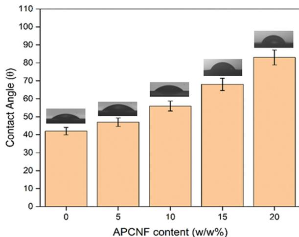
Fig. 11 Contact angle of APCNF-incorporated alginate films.
