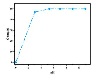
Fig. 5 Variation in the adsorption capacity of CV dye as a function of pH.
