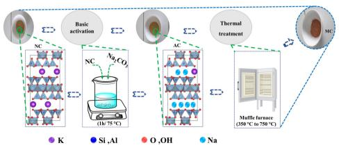
Fig. 1 Preparation of modified clays (MCs).
