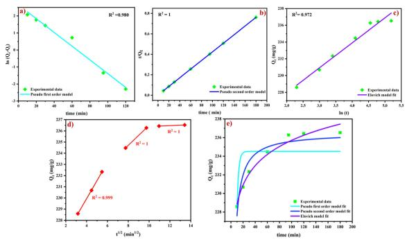
Linear regression of PSF (a), PSO (b), Elovich (c), and IPD (d) models and (e) nonlinear regression models for CV dye adsorption on AC-750 °C.
