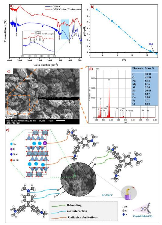
Fig. 11 FTIR spectra of (a) AC-750 °C and AC-750 °C@CV, pH<sub>pzc</sub> of (b) AC-750 °C, SEM images (c) and EDS analysis (d) of AC-750 °C@CV, and graphical illustration (e) of CV dye removal using AC-750 °C.
