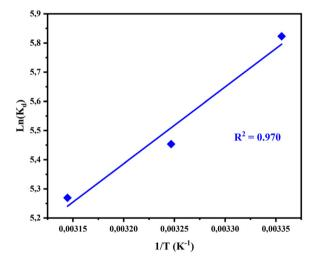
Van't Hoff plot for CV dye adsorption onto AC-750 °C
