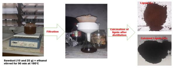
Fig. 1 Schematic of lignin extraction.
