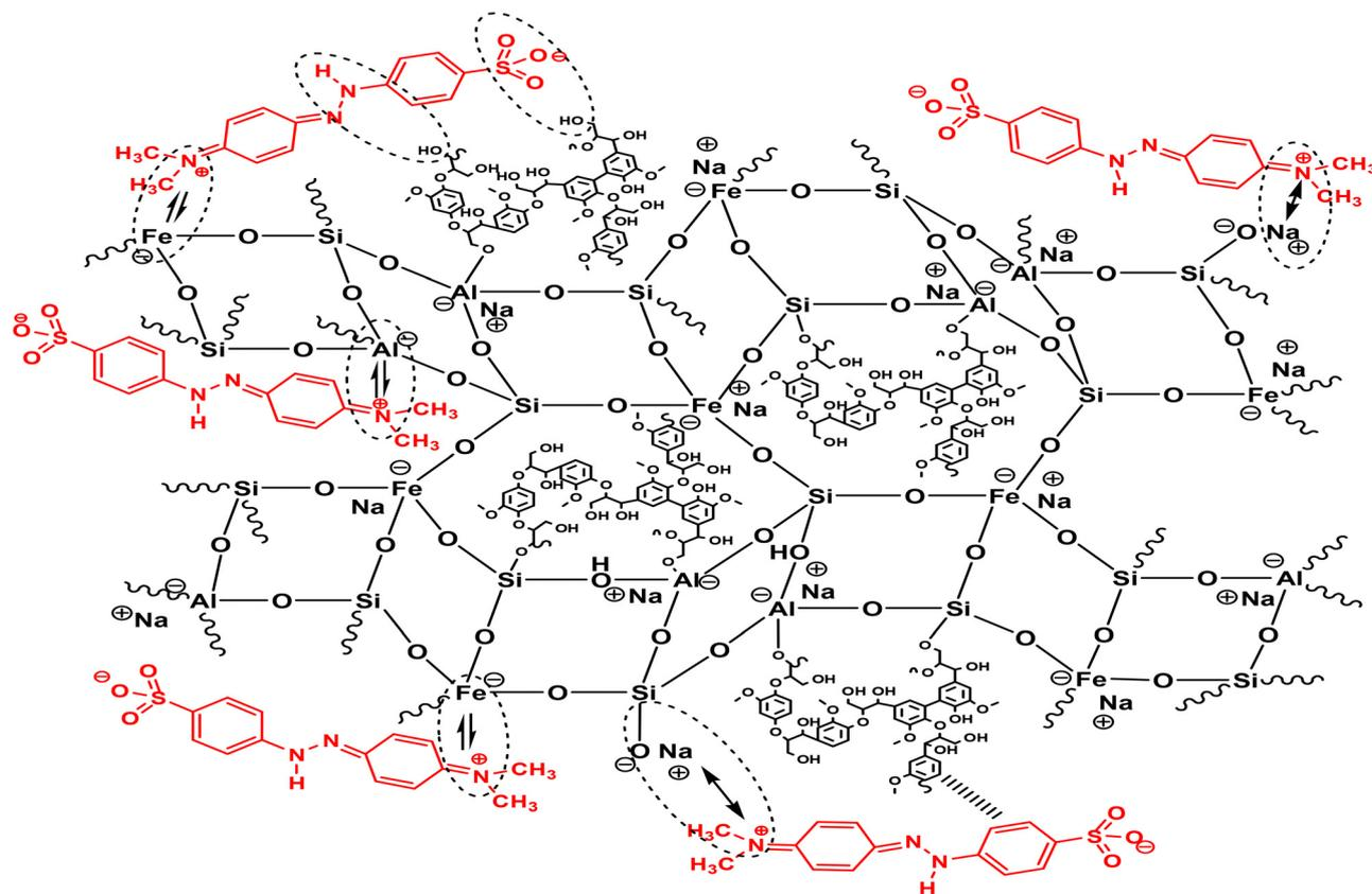
Fig. 14 Adsorption mechanism of MO on the geopolymer–lignin composite.
