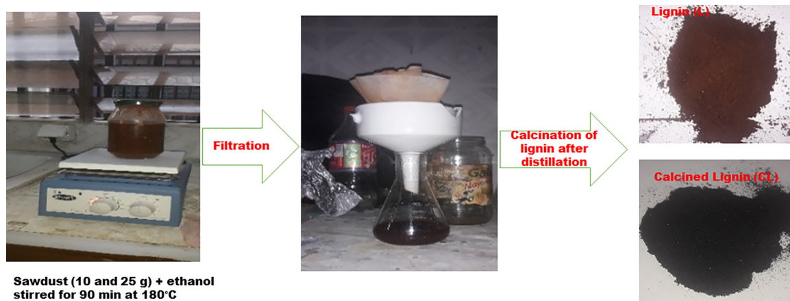
Fig. 1 Schematic of lignin extraction.
