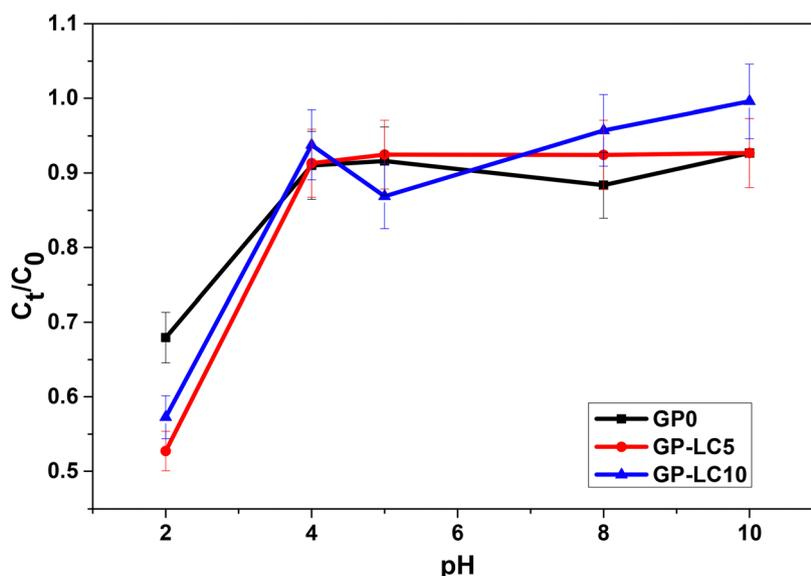
Fig. 10 Effect of pH on the adsorption of MO by GP0, GP-CL5 and GP-CL10 materials ( $m = 0.4$  g,  $C_0 = 10$  mg L<sup>-1</sup>).
