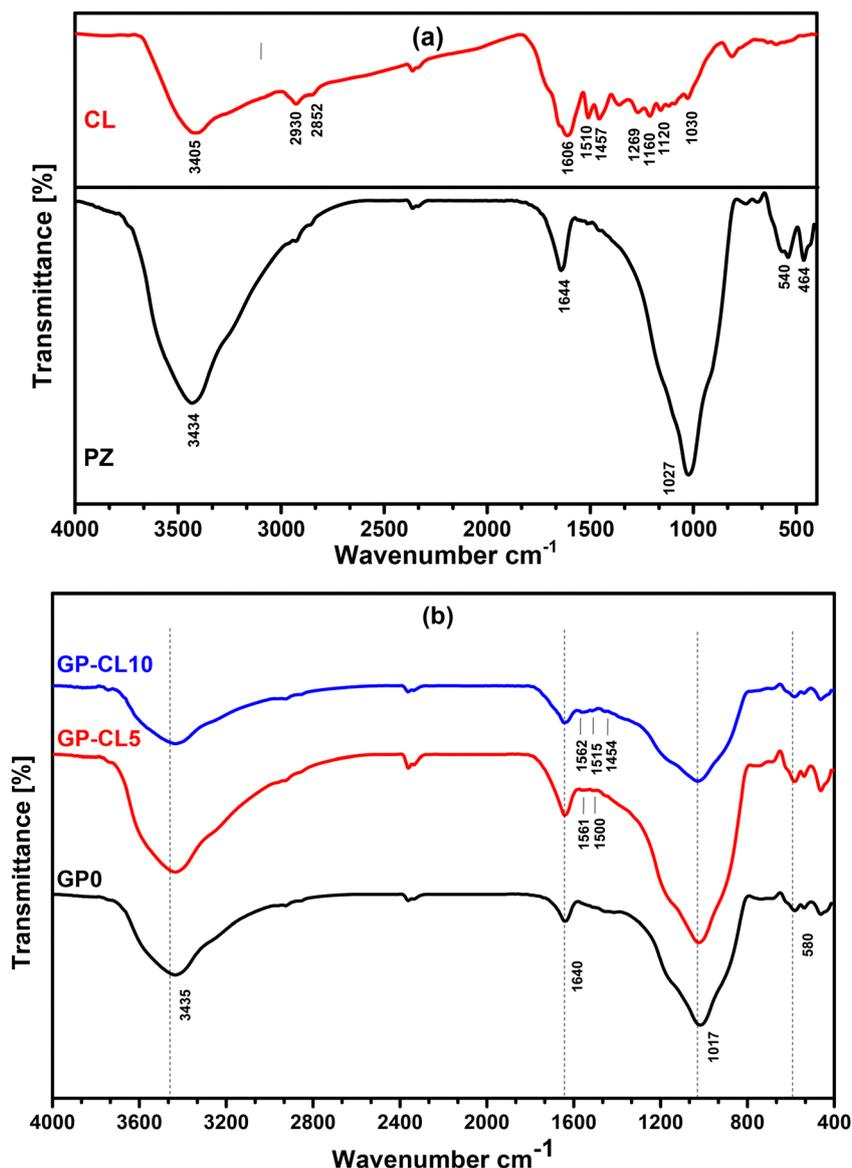
Fig. 6 FTIR spectra of precursors (a) and geomaterials (b).
