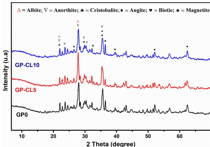
Fig. 5 XRD patterns of GP0, GP-CL5 and GP-CL10.
