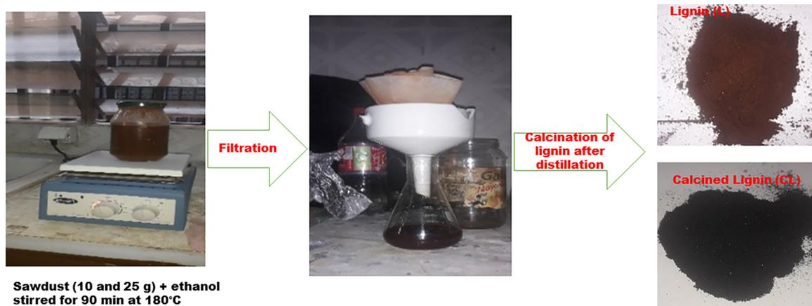
Fig. 1 Schematic of lignin extraction.
