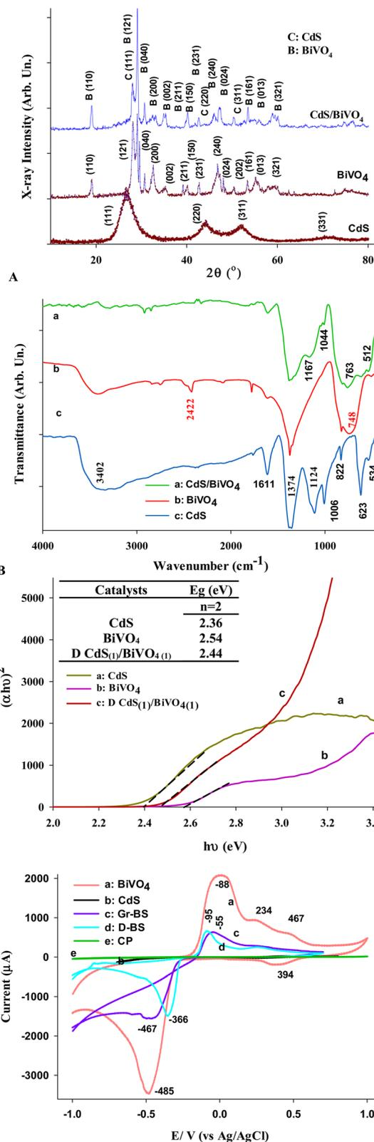
Fig. 1 XRD patterns (A), FTIR spectra (B),<sup>60,61</sup> typical Tauc plots (C), and CVs (D) for the individual and coupled samples.
