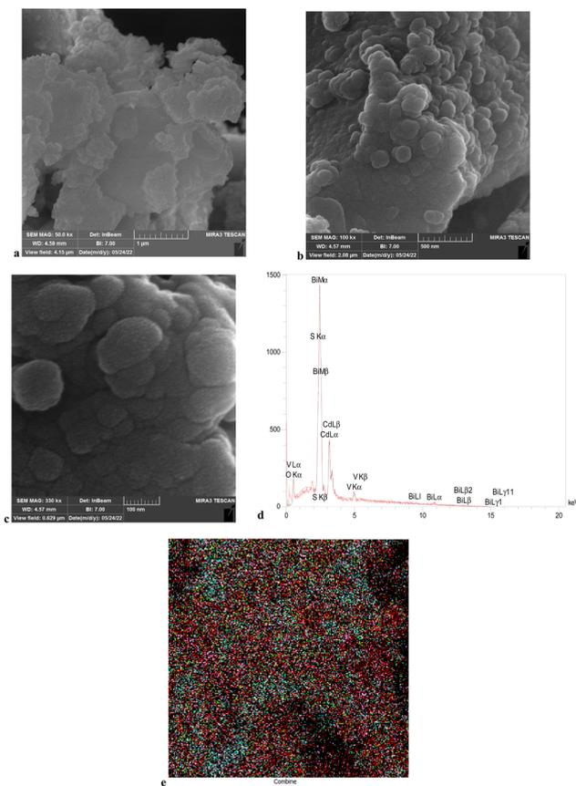
Fig. 2 SEM (A)–(C), EDX spectrum (D), and typical X-ray map (E) for the deposition prepared CdS/BiVO<sub>4</sub>.<sup>60,61</sup>
