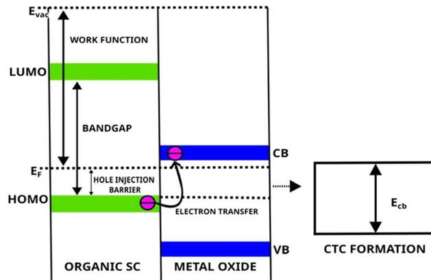
Fig. 2 Schematic representation of the charge transport complex between a metal oxide and an organic semiconductor.
