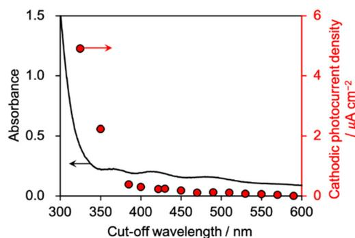
Fig. 4 Dependence of the cathodic photocurrent density of the PrCrO<sub>3</sub> thin film photocathode on the cut-off wavelength of the incident light. Light source: a 300 W Xe-arc lamp equipped with the corresponding cut-off filters (namely, long pass filters), electrolyte: an aqueous K<sub>2</sub>SO<sub>4</sub> solution containing phthalate buffer (pH4) saturated with Ar, applied potential:  $-0.4$  V vs. RHE, electrode area: approximately 1 cm<sup>2</sup>.
