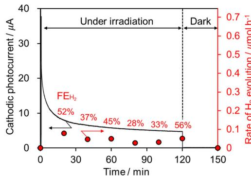
Fig. 5 Photoelectrochemical H<sub>2</sub> production using the PrCrO<sub>3</sub> thin film photocathode under UV irradiation. Light source: a 300 W Xe-arc lamp ( $\lambda > 300$  nm), electrolyte: an aqueous K<sub>2</sub>SO<sub>4</sub> solution containing phosphate buffer (pH7) saturated with Ar, applied potential: 0 V vs. RHE, electrode area: approximately 6 cm<sup>2</sup>.
