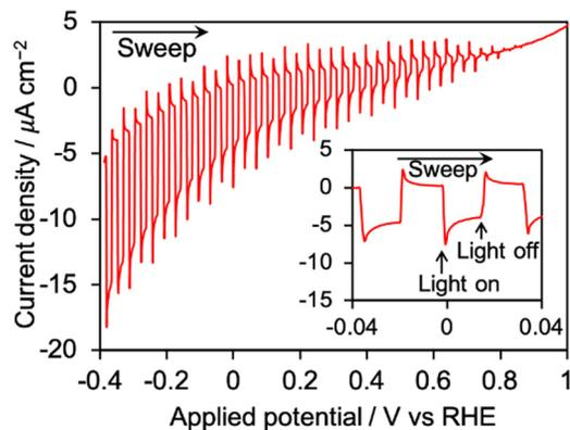
Fig. 3 Linear sweep voltammogram of the PrCrO<sub>3</sub> thin film photocathode. The inset figure is the magnified image of the area around 0 V vs. RHE. Light source: a 300 W Xe-arc lamp ( $\lambda > 300$  nm), electrolyte: an aqueous K<sub>2</sub>SO<sub>4</sub> solution containing phosphate buffer (pH7) saturated with Ar, electrode area: approximately 1 cm<sup>2</sup>.
