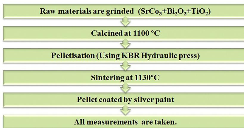
Fig. 1 Synthesis process of the sample.
