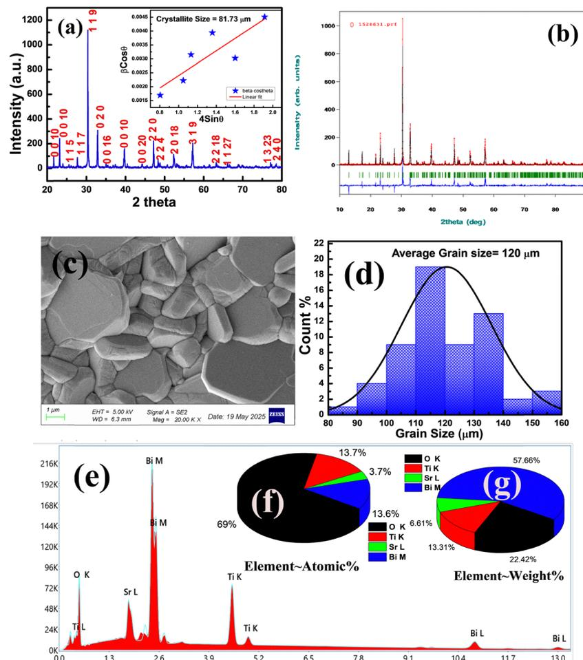
Fig. 2 (a) X-ray diffraction pattern of SBT, (b) Rietveld refinement, (c) FESEM micrograph of the compound SBT, (d) histogram plot of grain size, (e) EDX spectrum, and (f) and (g) pie chart of element versus atomic percentage and weight percentage.
