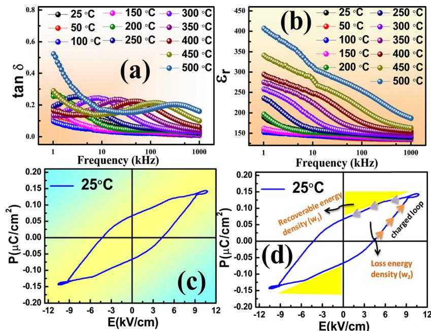
**Fig. 3** (a) Dielectric constant as a function of temperature for various frequencies, (b) dielectric loss as a function of temperature for various frequencies, (c) at 25 °C, ferroelectric  $P$ – $E$  hysteresis loop for SBT, and (d) energy storage density from the polarisation study.
