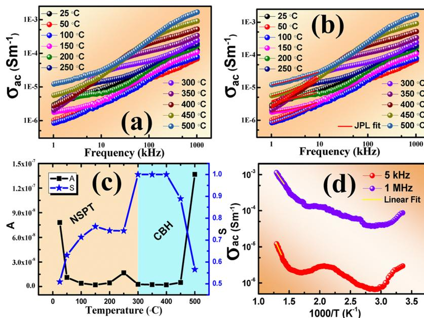
Fig. 6 (a) Depicts the variation of the ac conductivity of the sample with respect to the frequency, (b) JPL fitting, (c) the temperature response of  $s$  and  $A$  and (d) the variation of the ac conductivity of the sample with respect to the temperature.
