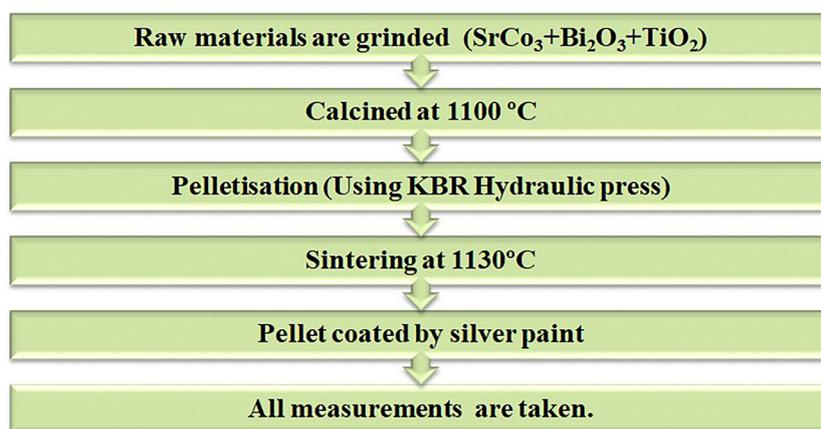
Fig. 1 Synthesis process of the sample.
