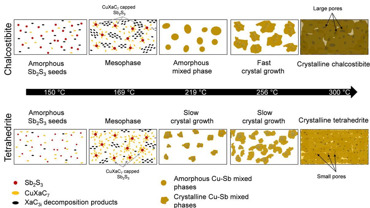
Fig. 6 Schematic illustration of the formation of the chalcostibite and tetrahedrite films based on the time resolved X-ray scattering and TEM characterizations.
