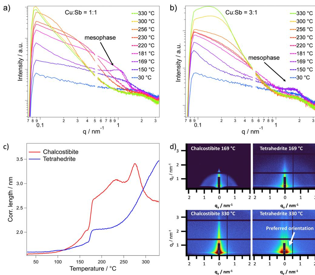
**Fig. 3** In-plane GISAXS scattering curves at selected temperatures during the heating runs of (a) chalcostibite and (b) tetrahedrite thin films; (c) in-plane correlation length derived from the GISAXS data in a  $q$  range of  $q = 0.08$  to  $q = 3.27 \text{ nm}^{-1}$ , and (d) 2D GISAXS images (left chalcostibite, right tetrahedrite) at 169 °C (top) and at 330 °C (bottom).
