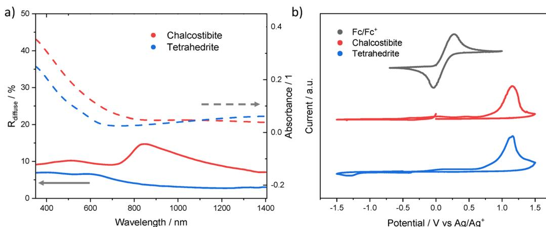
**Fig. 2** (a) Absorbance and diffuse reflectance spectra of chalcocite and tetrahedrite films on glass; (b) cyclic voltammograms of chalcocite (red) and tetrahedrite (blue) films with ferrocene (grey) as external standard.
