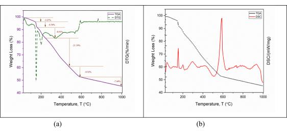
Thermal behavior of the CoFe<sub>2</sub>O<sub>4</sub> sample before calcination (for the sol gel method) (a) DTG and (b) DSC.
