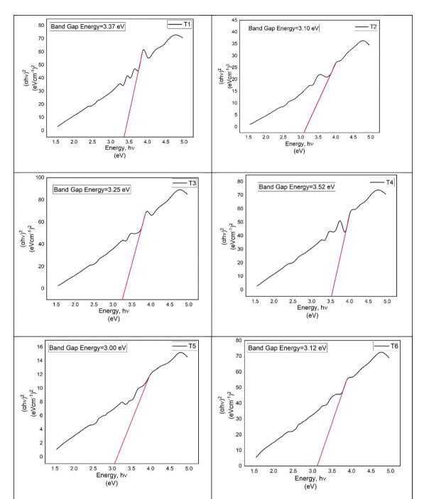
Fig. 12 Band gap energy of cobalt ferrite (CFO) NPs (T1, T2, T3, T4, T5 and T6).
