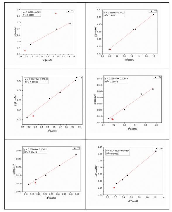
Fig. 5 SSP plot of cobalt ferrite for different calcination temperatures.
