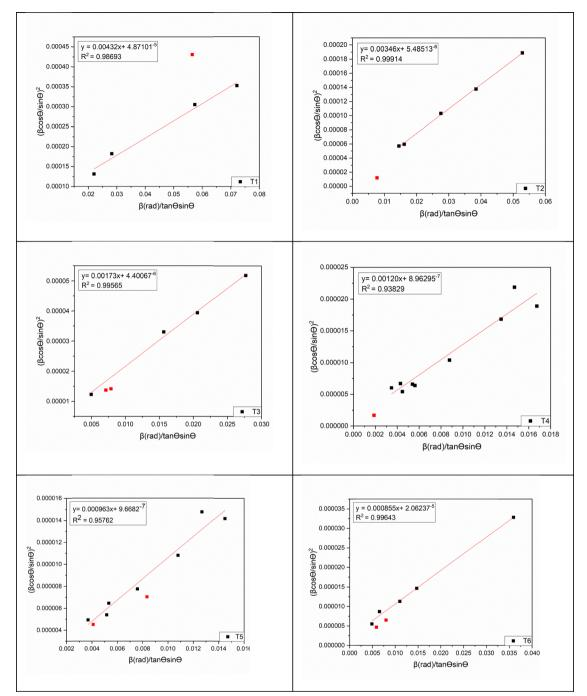
Fig. 4 H–W plot of cobalt ferrite nanoparticles (for different calcination temperatures)
