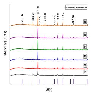
Fig. 2 XRD patterns of CFO nanoparticles calcined at 500  $^{\circ}$ C, 600  $^{\circ}$ C, 700  $^{\circ}$ C, 800  $^{\circ}$ C, 900  $^{\circ}$ C and 1000  $^{\circ}$ C with the standard XRD pattern of CFO.
