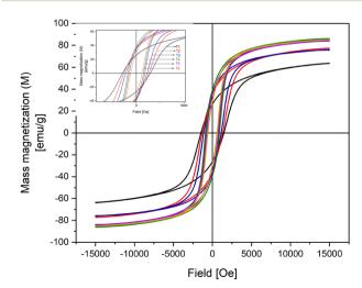
Fig. 7 M-H curves measured at room temperature for CoFe<sub>2</sub>O<sub>4</sub> samples
