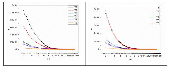
Fig. 10 Dielectric constant ( $\varepsilon' + \varepsilon''$ ) behaviour of the samples in the frequency range 20 kHz to 20 MHz.
