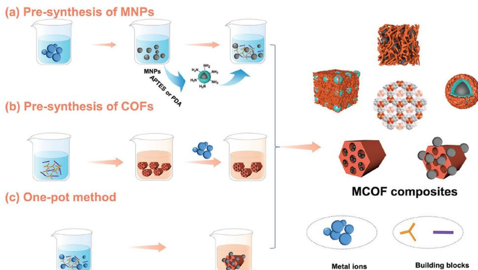
Fig. 6 The general preparation procedures of magnetic COFs.<sup>42</sup> Copyright 2023, Wiley.
