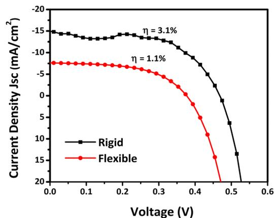
Fig. 6  $J$ - $V$  curves of the APPJ-printed CZTS-based solar cells on rigid and flexible substrates, measured under light illumination ( $100 \text{ mW cm}^{-2}$ , AM 1.5).
