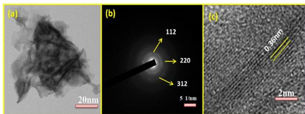
Fig. 4 (a) TEM image, (b) selected-area electron diffraction (SAED) pattern, and (c) HRTEM image of the APPJ-printed CZTS film.
