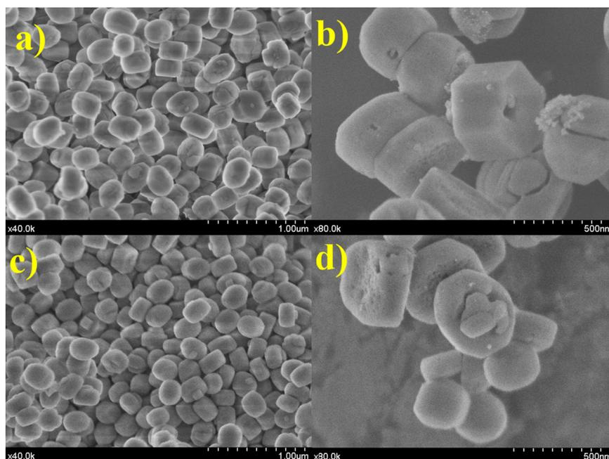
Fig. 5 SEM images of synthesized catalyst (a) TS<sub>20</sub> and (b) after its corresponding gold deposition; (c) synthesized TS<sub>80</sub> and (d) after its corresponding gold deposition.
