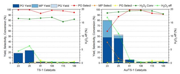
Fig. 8 Product distribution in propylene epoxidation reaction with TS\_X and Au/TS\_X catalysts. Reaction conditions: 150 mg catalyst, 10 mL methanol, 2.58 mL  $H_2O_2$  35% wt (30 mmol) and 4 bar propylene for 2 hours at 50 °C.
