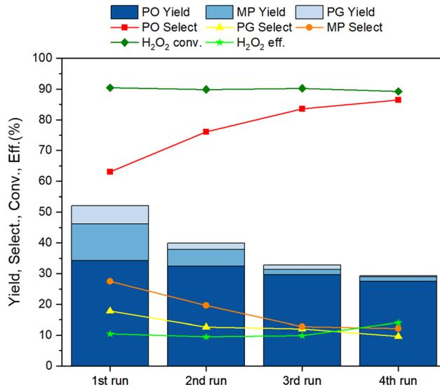
Fig. 10 Recyclability test in the propylene epoxidation reaction with the Au/TS<sub>30</sub> catalyst over 4 consecutive runs. Reaction conditions: 150 mg catalyst, 10 mL methanol, 2.58 mL H<sub>2</sub>O<sub>2</sub> 35 wt% (30 mmol) and 4 bar propylene for 4 hours at 50 °C.
