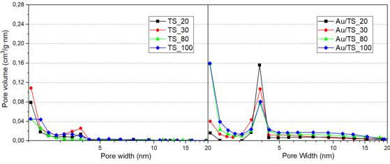
Fig. 4 Pore size distribution of representative TS\_X and Au/TS\_X samples.
