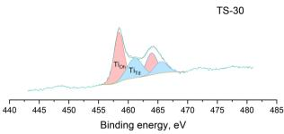
Fig. 7 Ti 2p high resolution XPS spectra of TS\_30 and Au/TS\_30 samples.
