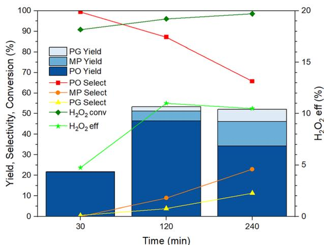
Fig. 9 Product distribution evolution over time in propylene epoxidation reaction with Au/TS<sub>30</sub> catalyst. Reaction conditions: 150 mg catalyst, 10 mL methanol, 2.58 mL H<sub>2</sub>O<sub>2</sub> 35% wt (30 mmol) and 4 bar propylene at 50 °C for different time periods.
