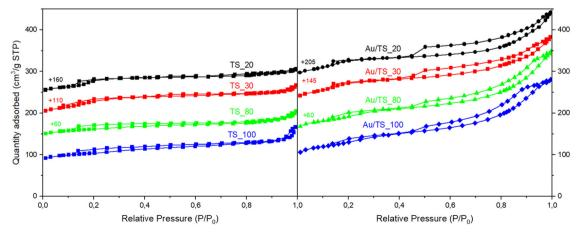
Fig. 3 N<sub>2</sub> adsorption-desorption isotherms at 77 K for the TS\_X and Au/TS\_X catalysts.
