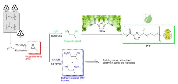
Fig. 1 Obtention of propylene glycol through HPPO route and posterior polymerization with FDCA to produce PEF.
