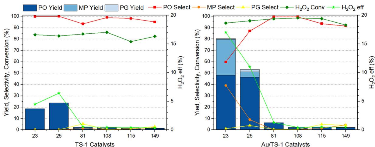
Fig. 8 Product distribution in propylene epoxidation reaction with TS\_X and Au/TS\_X catalysts. Reaction conditions: 150 mg catalyst, 10 mL methanol, 2.58 mL  $H_2O_2$  35% wt (30 mmol) and 4 bar propylene for 2 hours at 50 °C.
