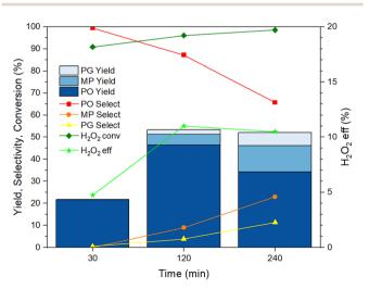
Fig. 9 Product distribution evolution over time in propylene epoxidation reaction with Au/TS\_30 catalyst. Reaction conditions: 150 mg catalyst, 10 mL methanol, 2.58 mL  $H_2O_2$  35% wt (30 mmol) and 4 bar propylene at 50 °C for different time periods.
