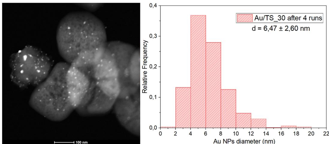
Fig. 11 Representative TEM image with HAADF detector of the Au/TS<sub>30</sub> catalyst after 4 epoxidation runs and its respective gold nanoparticle size-distribution histogram.
