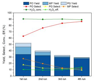
Fig. 10 Recyclability test in the propylene epoxidation reaction with the Au/TS\_30 catalyst over 4 consecutive runs. Reaction conditions: 150 mg catalyst, 10 mL methanol, 2.58 mL H<sub>2</sub>O<sub>2</sub> 35 wt% (30 mmol) and 4 bar propylene for 4 hours at 50 °C
