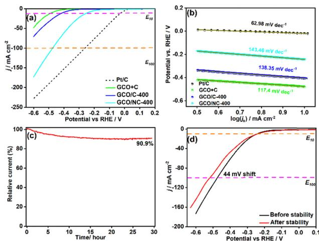
Fig. 7 (a) The LSVs of the synthesized electrocatalysts in the HER region (0 to  $-0.6$  V) in 1 M KOH as the electrolyte and at  $10 \text{ mV s}^{-1}$  as the scan rate, and 2000 rpm rotational speed, (b) the Tafel plots with slopes, (c) the stability (chronoamperometry) of GCO/NC-400 at a constant potential ( $-0.24$  V, where the current density reaches  $10 \text{ mA cm}^{-2}$ ), and (d) comparison of HER activity before and after the stability test.
