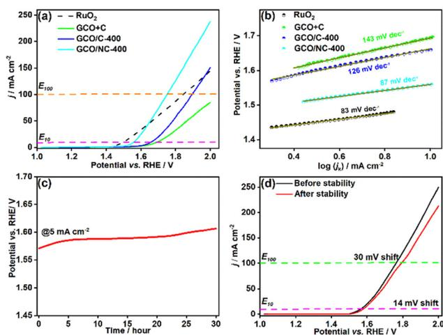
**Fig. 5** (a) OER activity of Gd and/or cobalt-based compounds in 1 M KOH as the electrolyte at a scan rate of 10  $\text{mV s}^{-1}$  at a rotational speed of 2000 rpm, and (b) the corresponding calculated Tafel slopes using kinetic current. (c) chronopotentiometry stability test of GCO/NC-400 at the current density of 5  $\text{mA cm}^{-2}$  and the rotational speed of 2000 rpm. (d) RDE LSV before and after the stability test.
