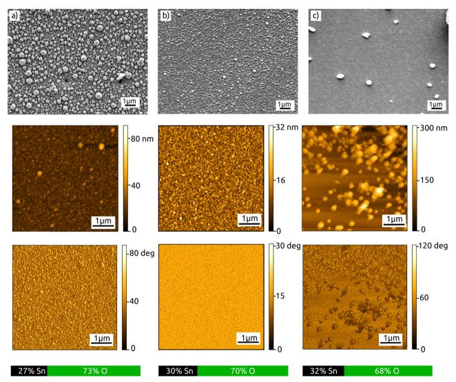
Fig. 4 Morphology characterization of the ALAM-deposited SnO<sub>2</sub> material. Top, scanning electron micrographs (10k magnification); center, topography, atomic force micrographs (5  $\times$  5  $\mu$ m<sup>2</sup>); lower line, atomic force micrographs phase image and EDX analyses (bar graphs at bottom). The 3 columns represent results obtained with deposition at 150 °C (a), 200 °C (b) and 250 °C (c), 400 passes all.
