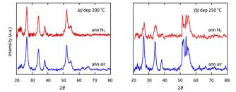
Fig. 5 X-ray diffraction data collected in grazing incidence geometry for ALAM-deposited  $SnO_2$  squares (3  $\times$  3 mm<sup>2</sup>, 400 passes) deposited at various temperatures, after annealing at 500 °C in nitrogen (red) or air (blue).
