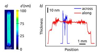
Fig. 3 (a) Thickness map measured by imaging ellipsometry of an ALAMprinted SnO<sub>2</sub> line (200 passes, 200 °C). (b) Thickness profiles extracted from (a) along the length of the line (red curve) and perpendicular to it (blue curve). The thickness shows a standard deviation of 1.4 nm along the 1521 data points in the central section of the length profile.
