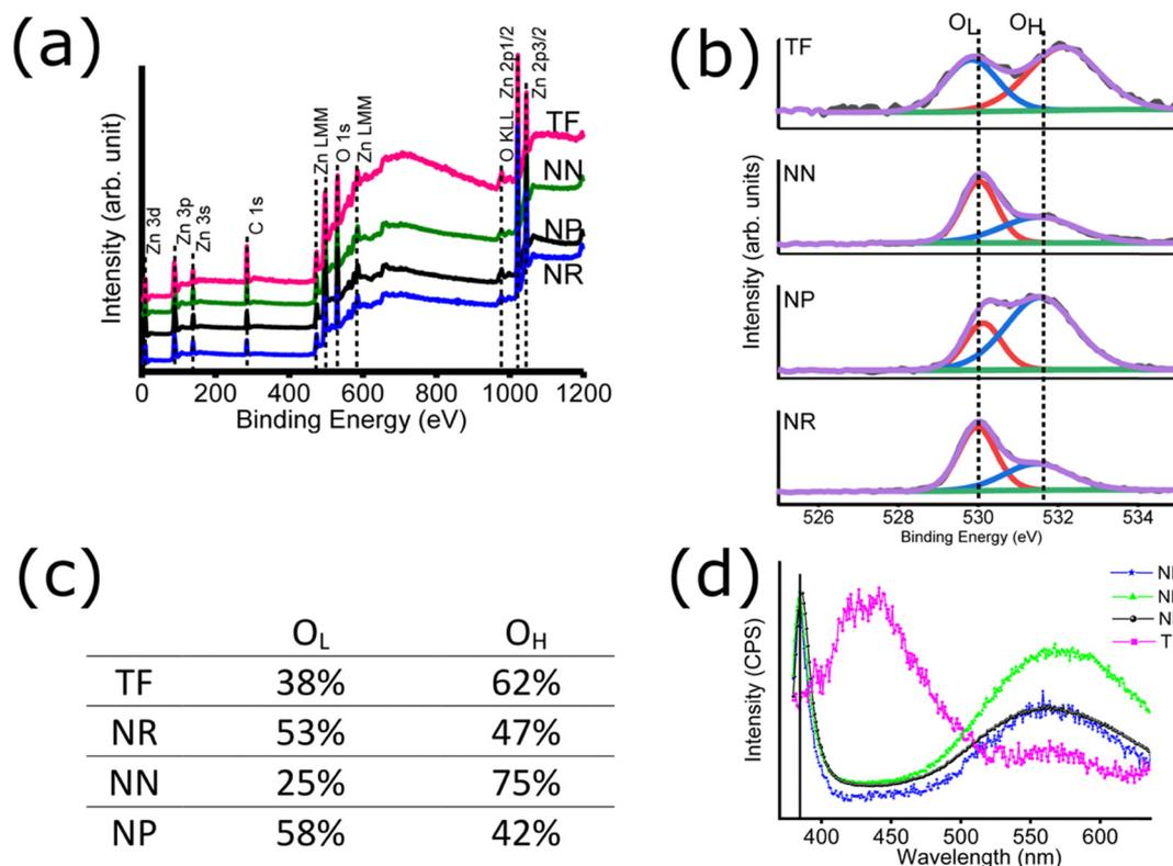
Fig. 4 Surface chemical composition of the ZnO coatings and photoluminescence spectra. (a) XPS spectra; (b) decomposition and (c) results of the approximate surface percentage of O<sub>L</sub> and O<sub>H</sub> of the O 1s peaks of ZnO TF, NN, NP, and NR coatings; and (d) normalized (to near band edge emission) room temperature photoluminescence spectra.
