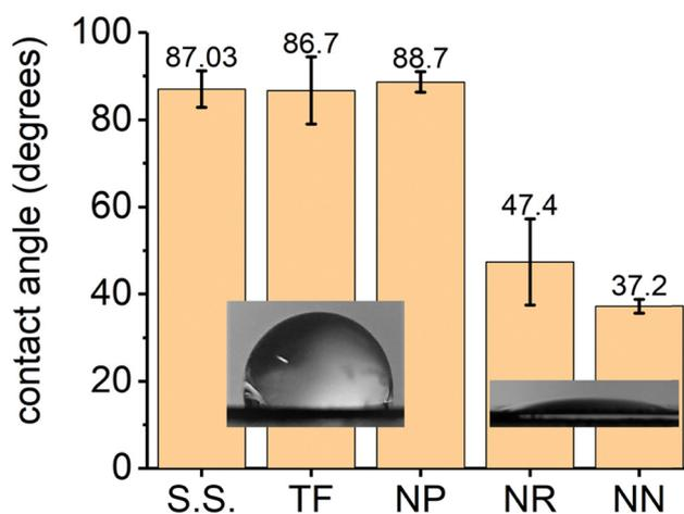
**Fig. 3** Wettability of the ZnO coatings. Contact angle ( $\theta$ ) formed by a 5- $\mu\text{L}$  water droplet on ZnO coatings with different topologies. Data presented as average  $\pm$  SD ( $n = 4$ ; *i.e.*, 4 drops on 4 different spots of the same coupon).
