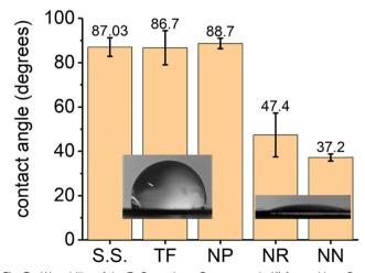
Fig. 3 Wettability of the ZnO coatings. Contact angle ( $\theta$ ) formed by a 5- $\mu$ L water droplet on ZnO coatings with different topologies. Data presented as average  $\pm$  SD (n = 4; i.e., 4 drops on 4 different spots of the same coupon).
