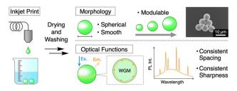
Fig. 1 Schematic illustration of the inkiet printing method for the fabrication of spherical polymer particles with monodisperse and modulable size distribution. The particles exhibit whispering gallery mode (WGM) optical resonance and periodic sharp peaks in the emission spectrum.
