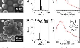
Fig. 4 Scanning electron micrographs (a) and (b), histograms of D (n = 205) (c) and (d), and microscopic photoluminescence spectra ( $\mu$ -PL,  $\lambda_{ex}$  = 450 nm) (e) and (f) of polymethyl methacrylate (PMMA), (a), (c) and (e) and polyvinylcarbazole (PVK), and (b), (d) and (f) microspheres produced from C<sub>2</sub>H<sub>4</sub>Cl<sub>2</sub> solutions (2 mg mL<sup>-1</sup>) through the inkjet printing
