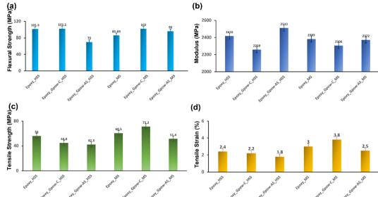
Fig. 4 Mechanical characteristics (a) flexural strength (MPa), (b) modulus (MPa), (c) tensile strength (MPa), and (d) tensile strain (%) of epoxy, GF and GNFbased composites with the variation of high-speed shearing (HSS) and mechanical stirring (MS); (three samples were tested and taking the average for each method).
