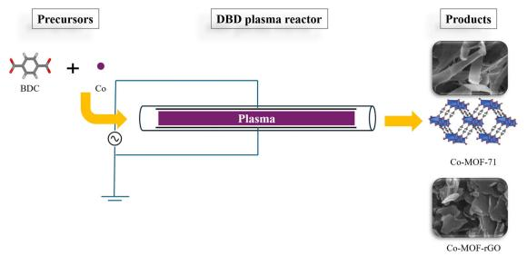
MOF composites synthesis process schematic by DBD plasma reactor. Reproduced from ref. 52 with permission from Nature Portfolio, copyright 2023.
