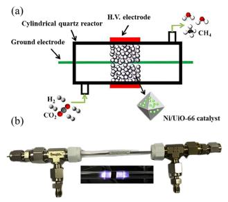
Fig. 10 (a) Schematic of DBD reactor and (b) photograph for the plasmacatalytic hydrogenation of CO<sub>2</sub>. Reproduced from ref. 100 with permission from John Wiley and Sons, copyright 2019.
