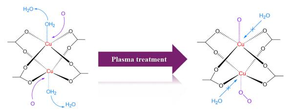
Fig. 7 Proposed O<sub>2</sub> plasma treatment mechanism of pore activation and protection. Reproduced from ref. 71 with permission from RSC, copyright 2017.
