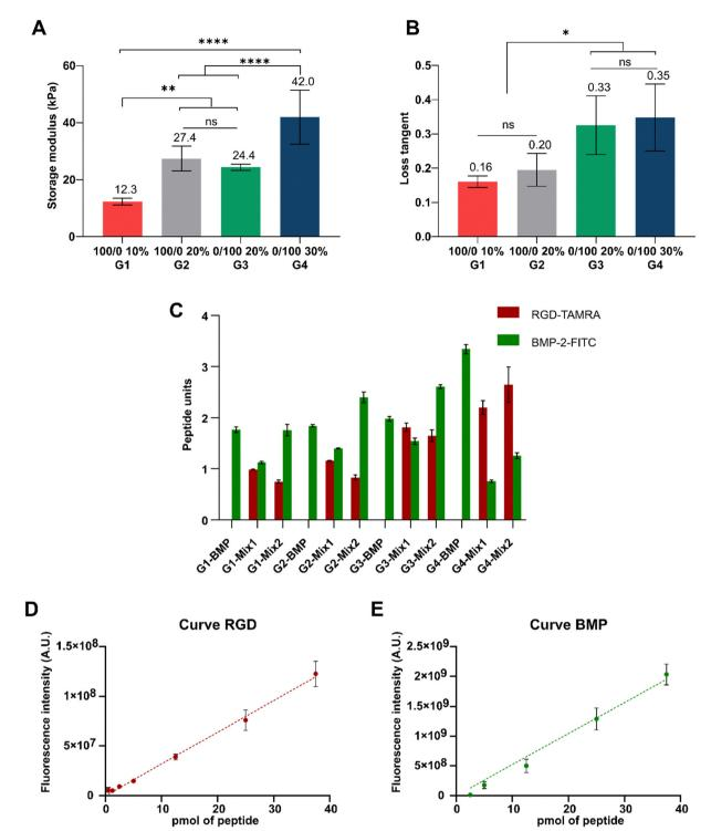
Fig. 1 Mechanical properties of PEGDA hydrogels measured by oscillatory rheology (n > 3). (A) Storage modulus and (B) loss tangent. Assessment of peptide density with fluorescence microscopy. (C) Calculated units of each peptide for the different hydrogel compositions (n = 3). Fluorescence calibration curves of RGD-TAMRA (D) and BMP-2-FITC (E).
