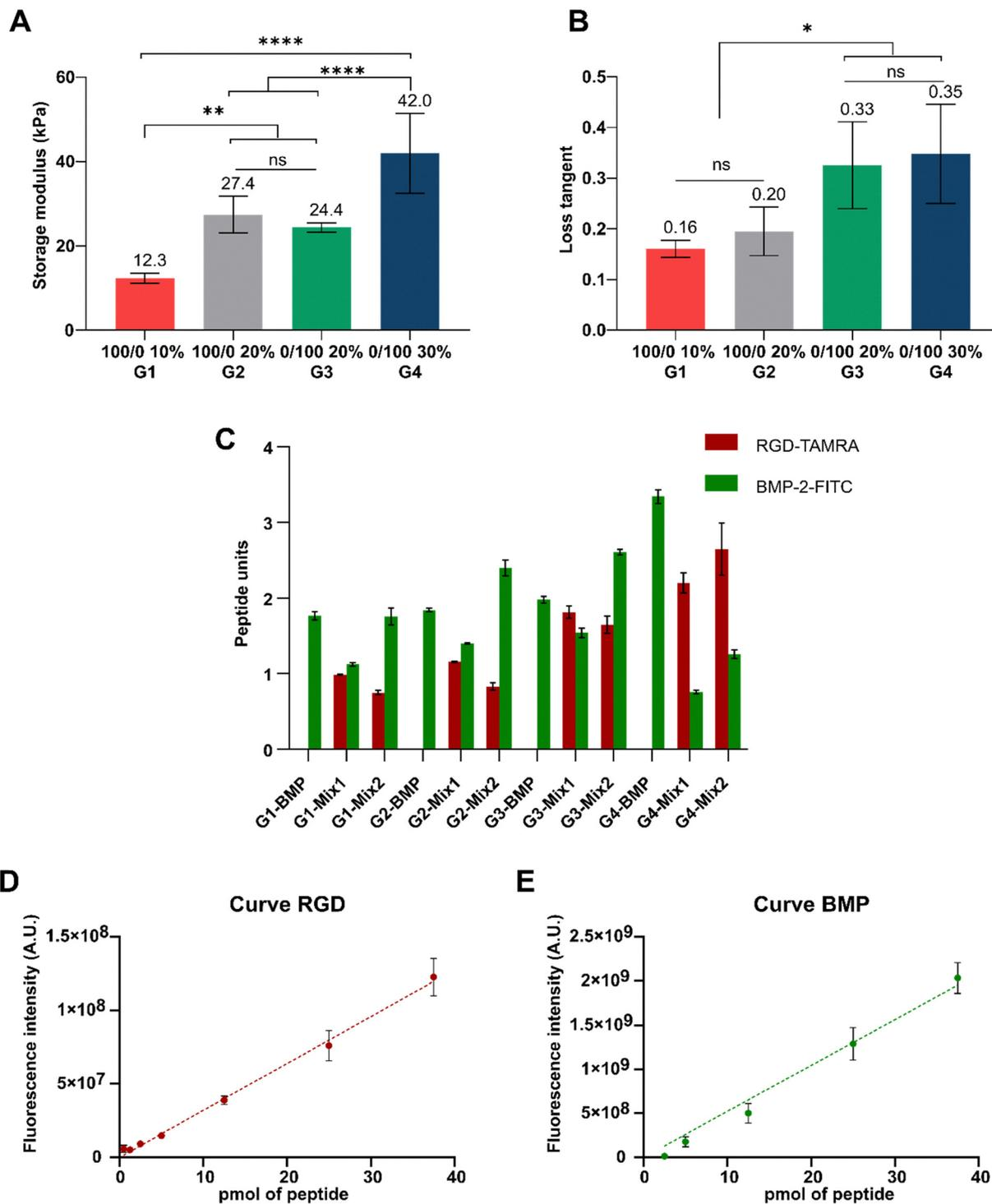
Fig. 1 Mechanical properties of PEGDA hydrogels measured by oscillatory rheology ( $n > 3$ ). (A) Storage modulus and (B) loss tangent. Assessment of peptide density with fluorescence microscopy. (C) Calculated units of each peptide for the different hydrogel compositions ( $n = 3$ ). Fluorescence calibration curves of RGD-TAMRA (D) and BMP-2-FITC (E).
