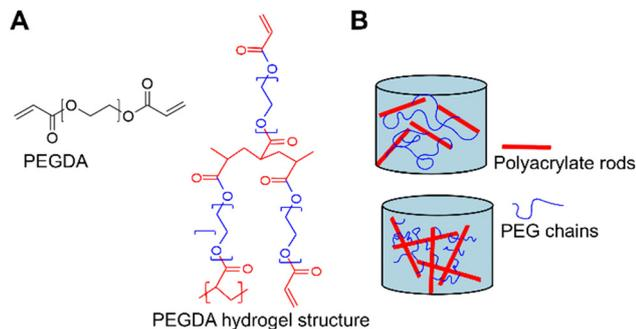
Fig. 4 Representative schematic of PEGDA hydrogel structure adapted from Levin *et al.*<sup>40</sup> (A) PEGDA oligomer structure and representation of the molecular organization with a polyacrylic backbone and connected PEGDA chains that, in turn, bind to other polyacrylate rods. (B) Schematic representation of two hydrogel compositions where  $\frac{L_{PEG}}{L_{PA}} > 1$  (top) and  $\frac{L_{PEG}}{L_{PA}} < 1$  (bottom).
