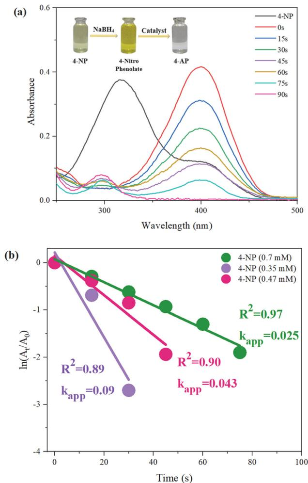
**Fig. 8** (a) Time-dependent UV-visible spectra of the reduction of 4-NP (0.7 mM) and (b) plot of  $\ln(A_t/A_0)$  versus time for the reduction of different 4-NP concentrations using  $\text{NaBH}_4$  (0.1 M). The mass of BCNF-CPTMS-Gu-Cu(II) was 0.01 g.
