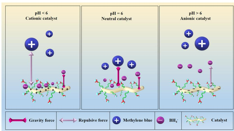
Fig. 11 Effect of ambient pH on the BCNF-CPTMS-Gu-Cu(II) catalyst in the MB reduction reaction.
