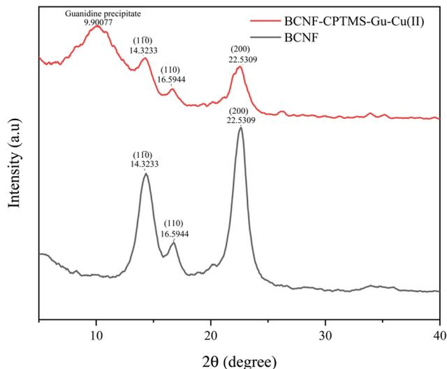
Fig. 4 XRD patterns of the BCNF and BCNF-CPTMS-Gu-Cu(II).
