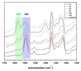
Fig. 5 Cutout of the IR spectra from functionalized PVBCB<sub>81</sub>-b-P4VPq $^{113k}_{19}$  membranes in the range of 1350-1700 cm $^{-1}$ . PVBCB<sub>81</sub>-b-P4VPq<sub>19</sub><sup>113k</sup> membranes after 1 h (red line), 2 h (red dotted line), 4 h (grey line), 8 h (grey dotted line), 16 h (dark grey line) and 24 h (dark grey dotted line) of functionalization with octylbromide as well as the pristine PVBCB<sub>81</sub>-b-P4VP<sub>19</sub><sup>113k</sup> membrane (black) are shown.
