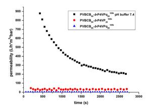
Fig. 8 Water flux measurements of block copolymer membranes  $PVBCB_{80}$ -b- $P4VP_{20}^{105k}$ ,  $PVBCB_{80}$ -b- $P4VPq_{20}^{105k}$  and  $PVBCB_{80}$ -b-P4VPq<sup>105k</sup> in PBS buffer with pH of 7.4.
