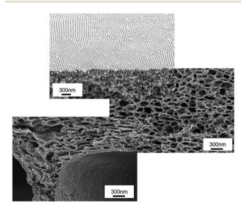
Fig. 7 SEM images of the cross-section of PVBCB<sub>80</sub>-b-P4VP<sup>105k</sup><sub>20</sub> block copolymer membrane showing the isoporous integral asymmetric structure
