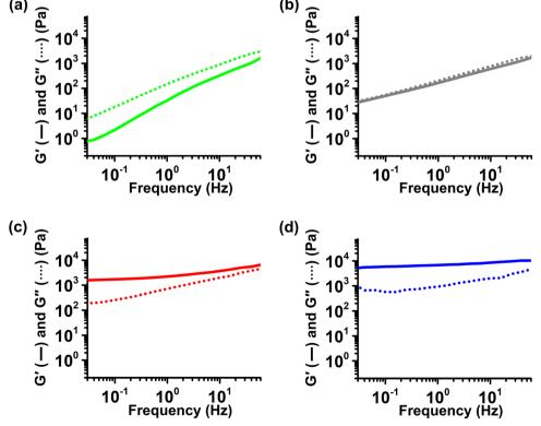
Fig. 4 Elastic (G') and viscous (G") moduli of Ga-in-glycerol emulsions with Ga contents of (a) 50 vol%, (b) 60 vol%, (c) 70 vol%, and (d) 80 vol%, obtained through frequency-sweep oscillatory rheological measurements under a constant stress of 1 Pa
