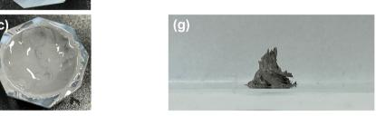
Fig. 1 Photographs of the emulsification products of Ga with glycerol solutions containing PVP concentrations of (a) 0 wt%, (b) 10 wt%, and (c) 20 wt% (Ga content: 50 vol%). Photographs of emulsification products prepared using a glycerol solution with 20 wt% PVP at varying Ga contents: (d) 60 vol%, (e) 70 vol%, and (f) 80 vol% Ga. (g) Photograph showing the state of the Ga-in-glycerol emulsion (80 vol% Ga) from (f) after 2 months of storage.
