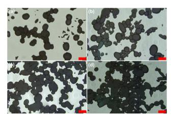
Fig. 2 Optical microscopy images of dispersed Ga particles in Ga-inglycerol emulsions with Ga contents of (a) 50 vol%, (b) 60 vol%, (c) 70 vol%, and (d) 80 vol%. The scale bars indicate 20  $\mu m$ .
