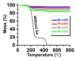
Fig. 3 TGA curves of the PCMEs with various Ga contents. The dashed line represents the data for the glycerol solution without Ga.
