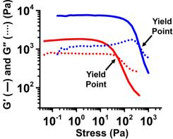
Fig. 5 Elastic (G') and viscous (G'') moduli of Ga-in-glycerol emulsions with Ga contents of 70 vol% (red) and 80 vol% (blue), obtained through stress sweep oscillatory rheological measurements under a constant frequency of 1 Hz.
