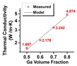
Fig. 7 Thermal conductivities of Ga-in-glycerol emulsions with various Ga contents. (Circled data points: measured values; dotted line: predicted by the Agari model).
