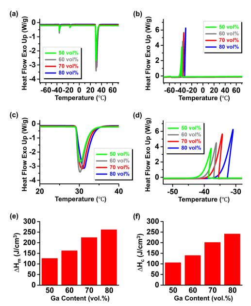
DSC (a) (c) heating and (b) (d) cooling curves of Ga-in-emulsions with various Ga contents. (e) Melting ( $\Delta H_{\rm m}$ ) and (f) crystallization ( $\Delta H_{\rm c}$ ) enthalpies of the respective Ga-in-glycerol emulsions
