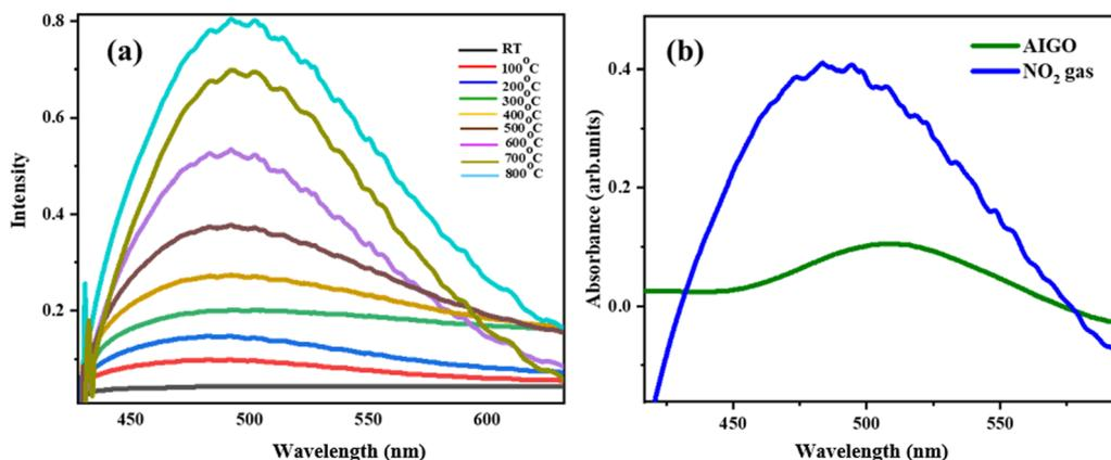
Fig. 6 (a) Absorbance of NO<sub>2</sub> gas as a function of temperature in the wavelength range of 450–600 nm and (b) superimposed optical absorbance of AIGO and NO<sub>2</sub> gas.
