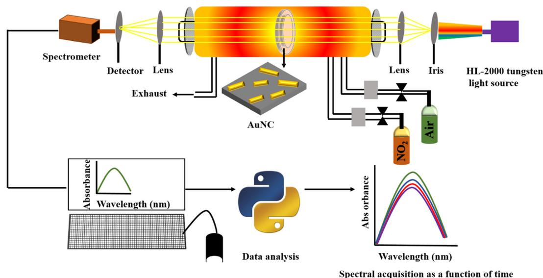
Fig. 2 Setup for optical sensing of  $\text{NO}_2$  at elevated temperatures, with mass flow controllers for regulating  $\text{NO}_2$  concentrations, a horizontal split-type furnace designed for optical measurements of samples in a ceramic holder, and optical elements such as collimators, plano-convex lenses, a light source, and a spectrometer.
