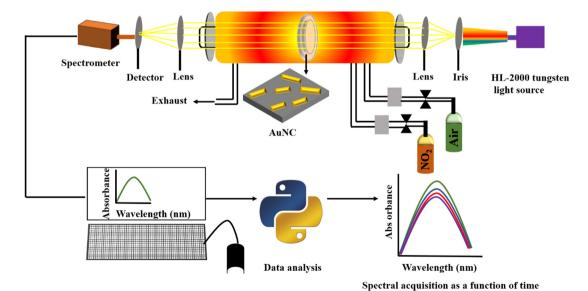
Fig. 2 Setup for optical sensing of NO<sub>2</sub> at elevated temperatures, with mass flow controllers for regulating NO<sub>2</sub> concentrations, a horizontal split-type furnace designed for optical measurements of samples in a ceramic holder, and optical elements such as collimators, plano-convex lenses, a light source, and a spectrometer.
