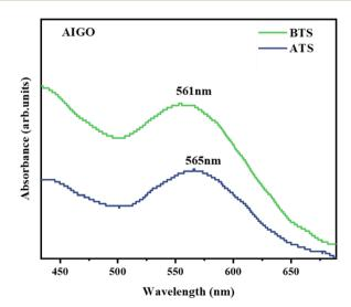
Fig. 3 Optical absorbance of the AIGO composite recorded before and after TS tests at room temperature. Reproduced with permission from ref. 30.
