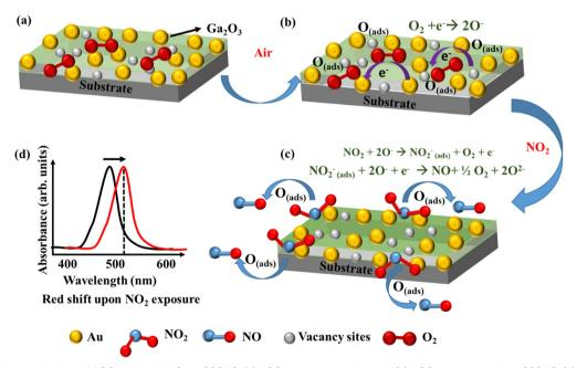
Fig. 10 Gas sensing mechanism of AGOs towards NO<sub>2</sub> at 800 °C: (a) AGO on a quartz substrate. (b) AGO exposed to air at 800 °C. (c) AGOs exposed to NO<sub>2</sub> in air background. (d) Shift towards the longer wavelength/redshift upon gas exposure.
