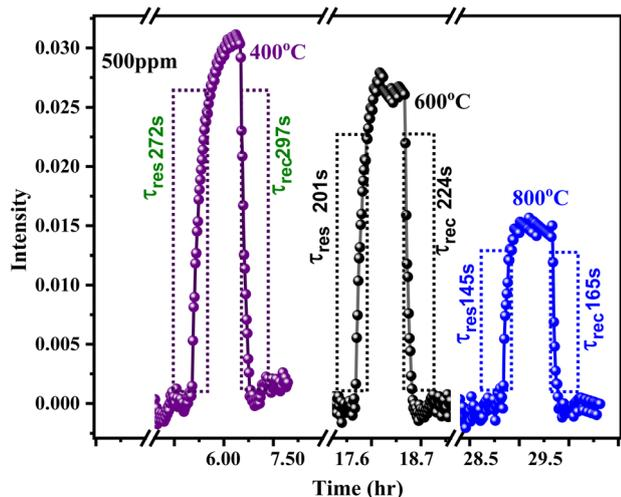
Fig. 11 Temperature-dependent sensing response of AIGO towards NO<sub>2</sub> at 500 ppm at different temperatures: 400 °C, 600 °C and 800 °C.
