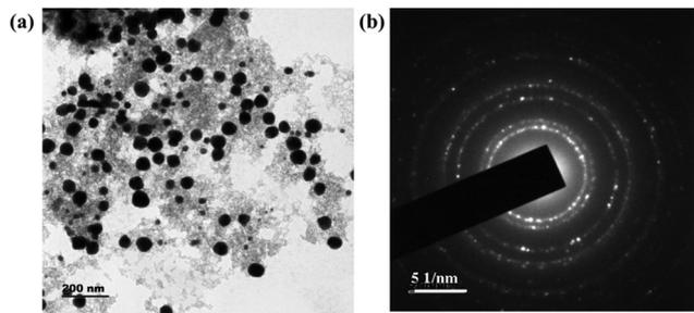
Fig. 5 (a) TEM images of the AIGO composite depicting the presence of Au and Ga<sub>2</sub>O<sub>3</sub>. (b) SAED diffraction pattern of AIGO with ring patterns and bright spots confirming the crystallinity of the composite. Reproduced with permission from ref. 28 and 30.
