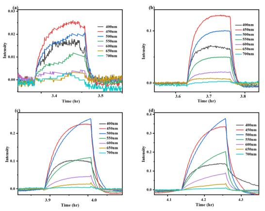
Fig. 8 Sensing responses of AIGO towards  $NO_2$  at 800 °C at concentrations of (a) 500 ppm, (b) 1000 ppm, (c) 2500 ppm and (d) 5000 ppm as a function of wavelength.
