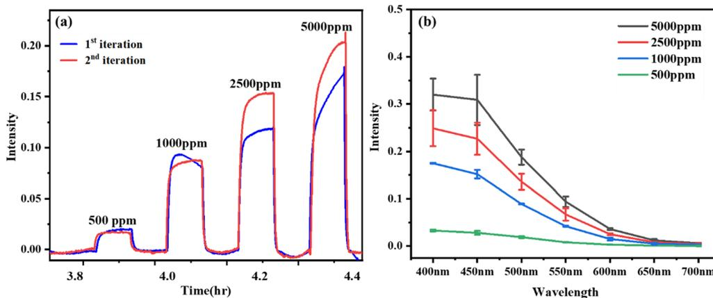
Fig. 7 (a) Intensity vs. time graph corresponding to NO<sub>2</sub> absorbance at 500 nm at various concentrations of 500 ppm, 1000 ppm, 2500 ppm and 5000 ppm recorded twice. (b) Standard deviation graph illustrating the intensity changes of the wavelengths in the range of 400–700 nm for all concentrations.
