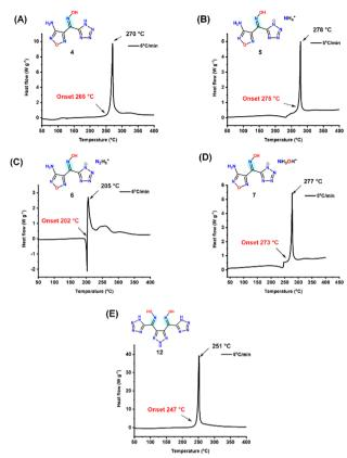
Fig. 4 DSC analysis at the heating rate of 5  $^{\circ}$ C min<sup>-1</sup> (A) **4**. (B) **5**. (C) **6**. (D) 7. (E) 12.
