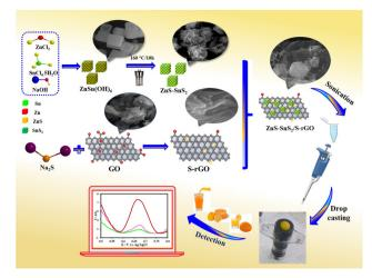
Scheme 1 Schematic illustration of ZnS-SnS<sub>2</sub>/S-rGO/CPE preparation for SY determination
