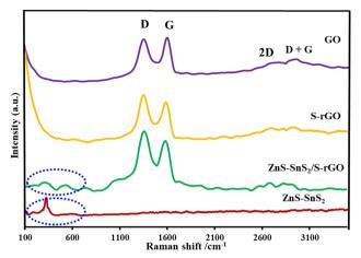
Fig. 6 Raman spectra of GO, S-rGO, ZnS-SnS<sub>2</sub>, and ZnS-SnS<sub>2</sub>/S-rGO
