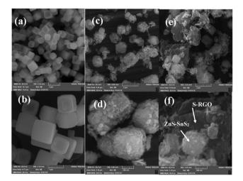
Fig. 1 FE-SEM images of (a) and (b) ZnSn(OH)<sub>6</sub> precursor, (c) and (d) ZnS-SnS<sub>2</sub>, and (e) and (f) ZnS-SnS<sub>2</sub>/S-rGO.
