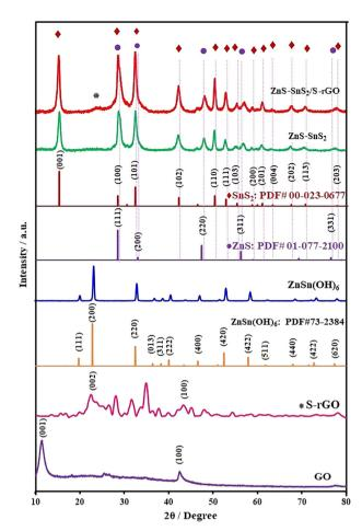
Fig. 3 XRD patterns of GO, S-rGO, ZnSn(OH)<sub>6</sub>, ZnS-SnS<sub>2</sub>, and ZnS-SnS<sub>2</sub>/ S-rGO.
