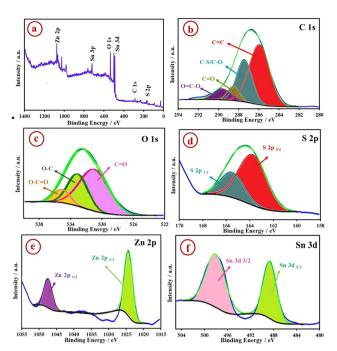
Fig. 4 The XPS (a) survey spectrum, (b) C 1s, (c) O 1s, (d) S 2p, (e) Zn 2p, and (f) Sn 3d high-resolution XPS spectra of the ZnS-SnS<sub>2</sub>/S-rGO.
