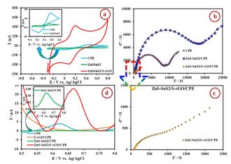
Fig. 7 (a) CVs, (b) and (c) Nyquist plots from  $10^5$  Hz to  $10^{-1}$  Hz frequencies in 0.1 M KCl solution containing 1.0 mM  $K_3Fe(CN)_6$ ; and (d) DPVs of 0.1 mM solution of the SY in 0.1 M PBS (pH = 7.5) at the GO, S-rGO, ZnS-SnS<sub>2</sub>, and ZnS-SnS<sub>2</sub>/S-rGO.
