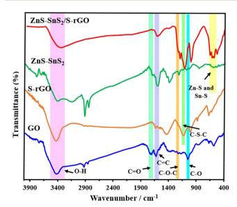
Fig. 5 FT-IR of GO, S-rGO, ZnS-SnS<sub>2</sub>, and ZnS-SnS<sub>2</sub>/S-rGO.
