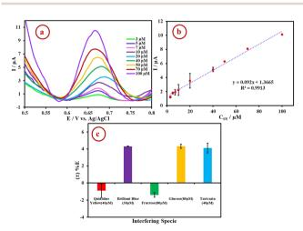
Fig. 9 (a) DPVs by increasing the concentration of SY from 3.0  $\mu M$  to 100  $\mu M$  in 0.1 M PBS solution (pH 7.5) at the ZnS-SnS2/S-rGO/CPE surface; (b) the calibration curve; (c) effect of various interferents on the SY sensing response of ZnS-SnS<sub>2</sub>/S-rGO/CPE. Error bars indicate the standard deviations of three repeated measurements.
