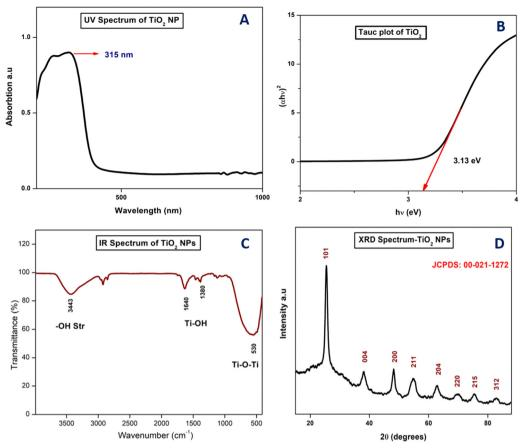
Fig. 1 (A) UV spectrum of the TiO<sub>2</sub> NPs. (B) Tauc plot for bandgap energy calculations. (C) FTIR spectrum of TiO<sub>2</sub> NPs. (D) XRD spectrum of TiO<sub>2</sub> NPs.
