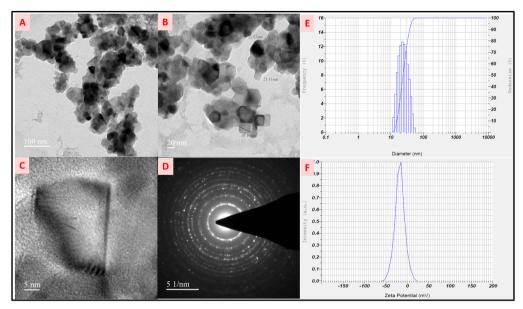
Fig. 3 (A)–(C) TEM images of the TiO<sub>2</sub> NPs. (D) SAED pattern. (E) Histogram of particle size analysis. (F) zeta potential distribution analysis of TiO<sub>2</sub>.
