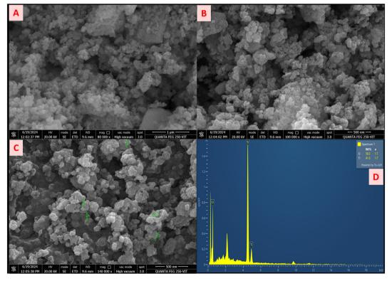
Fig. 2 (A)-(C) FESEM images of the TiO<sub>2</sub> NPs of different magnifications and (D) EDAX spectrum of the TiO<sub>2</sub> NPs
