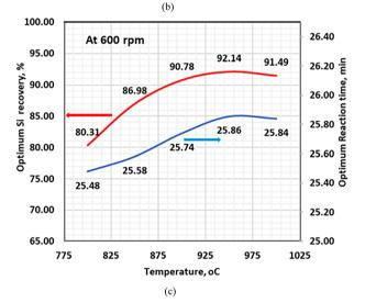
Fig. 7 Prediction of the minimum reaction time and the corresponding optimal value of Si recovery efficiency % at different temperatures at stirring speed: (a) 200 rpm, (b) 400 rpm and (c) 600 rpm.
