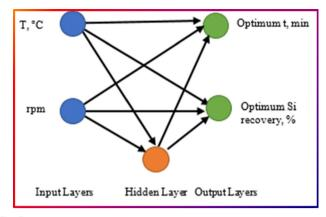
Fig. 3 The proposed ANN via the Levenberg-Marguardt algorithm to estimate the optimum reaction time corresponding to the maximum Si recovery efficiency
