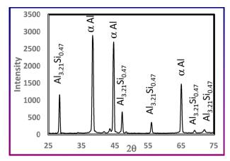
Fig. 4 XRD pattern of the produced Al-Si alloy produced by Na<sub>2</sub>SiF<sub>6</sub>
