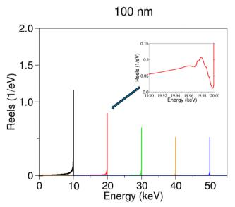
Fig. 5 Monte Carlo simulation of the reflection energy loss spectrum (Reels) of electrons emerging from a 100 nm thick CsPbBr<sub>3</sub> sample for different kinetic energies of the primary beam: 10 (black line), 20 (red line), 30 (green line), 40 (orange line) and 50 (blue line) keV. The inset shows the plasmon peak for a 20 keV electron beam
