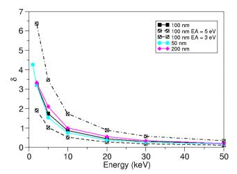
**Fig. 7** Reflection yield of the secondary electrons ( $\delta$ ) as a function of the kinetic energy of the primary beam (keV). The results are shown for three different sample thicknesses and electron affinities: 50 nm (cyan-coloured solid line), 100 nm (black solid line) and 200 nm (magenta-coloured solid line) for EA = 4.1 eV (pristine material). For the 100 nm layer, results with EA = 3.0 eV (black dash-dotted line) and 5.0 eV (black dashed line) are also included.
