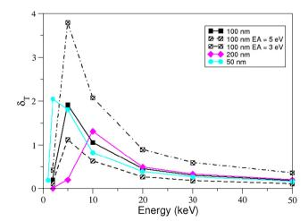
Fig. 10 Secondary electron transmission yield ( $\delta_T$ ) as a function of the initial kinetic energy of the primary beam (keV). The results are shown for three different sample thicknesses and electron affinities: pristine material (EA = 4.1 eV), 50 nm (cyan solid line), 100 nm (black solid line) and 200 nm (magenta solid line). The results for a depth of 100 nm with EA = 3.0 eV (black dashed line) and 5.0 eV (black dashed line) are also shown.
