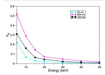
Fig. 6 Backscattering coefficient  $(\eta_B)$  for the electrons of the primary beam as a function of their initial kinetic energy (keV). The results are shown for three different sample thicknesses: 50 nm (cyan-coloured solid line), 100 nm (black solid line) and 200 nm (magenta-coloured solid line).
