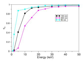
Fig. 9 Transmission coefficient ( $\eta_T$ ) for the primary electrons as a function of the initial electron kinetic energy (keV). The results are shown for three different sample thicknesses: 50 nm (cyan solid line), 100 nm (black solid line) and 200 nm (magenta solid line).
