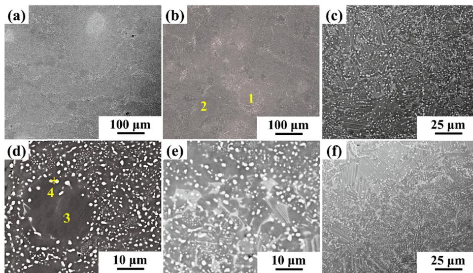
Fig. 9 Backscattered scanning electron microscopy of microstructures of samples after HIP and HT: (a) 80 W\_CH\_HIP\_1 sample along the longitudinal direction, (b) 100 W\_CH\_HIP\_1 sample along the longitudinal direction, (c) 100 W\_CH\_HIP\_2 sample along the transverse direction, (d) 100 W\_M\_HIP\_2 sample along the longitudinal direction, (e) 100 W\_M\_HIP\_2 sample along the transverse direction, and (f) 100 W\_CH\_HIP\_1 sample along the transverse direction.
