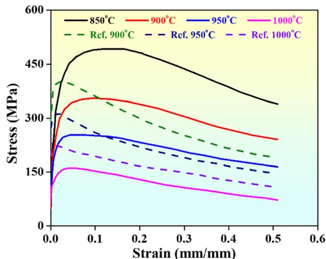
Fig. 11 Compressive true stress-true strain curves tested for the 80 W\_CH\_HIP\_1 + HT sample as a function of different testing temperatures and in comparison with Ti-43Al-8Nb-3.6C-0.7Mo tested under similar conditions.<sup>50</sup>
