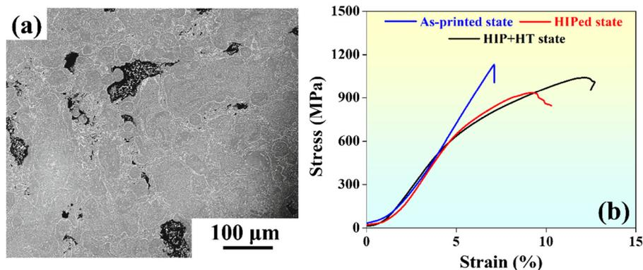
Fig. 16 (a) Backscattered scanning electron microscopy image of the 80 W\_CH sample along the transverse direction after application of HT and the subsequent HIP\_1 process. (b) Room temperature compressive stress–strain plot of the 80 W\_CH sample tested under different conditions.
