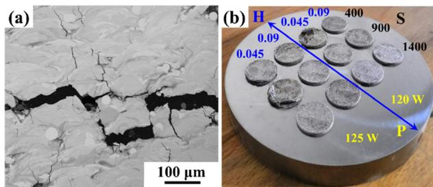
**Fig. 14** (a) Example of horizontal cracking in the sample after LPBF ( $P = 120$  W,  $S = 900$  mm  $s^{-1}$ ,  $h = 0.12$  mm, longitudinal cut (SEM/BSE). (b) Example of warping when inappropriate parameters are used during LPBF ( $h$  – hatch spacing (mm),  $v$  – scan speed (mm  $s^{-1}$ ),  $P$  – laser power).
