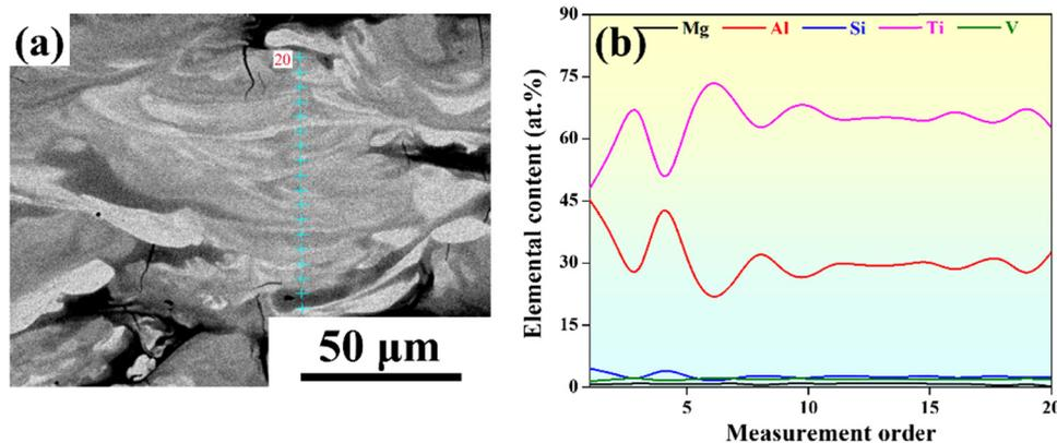
Fig. 12 (a) Micrograph showing the melt pool features observed in the LPBF 100 W\_CH sample along the longitudinal direction and (b) energy dispersive spectroscopy concentration profile showing the elemental distribution.
