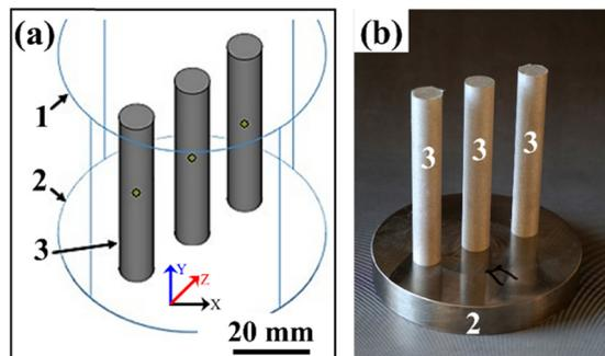
**Fig. 1** (a) The 3D print preview of samples in Materialise Magics software and (b) image of samples after 3D printing: (1) bounding box of the Trumpf TruPrint 1000 3D printer build area (blue lines), (2) substrate, and (3) vertical samples.
