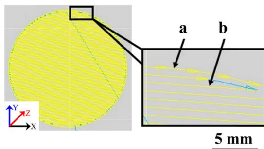
**Fig. 2** Schematics showing the details of the meander hatching strategy employed during the fabrication of the Ti–Al samples in the TruPrint 1000 3D printer. (a) The laser trajectory used at the contours and (b) the laser trajectory for the hatches.
