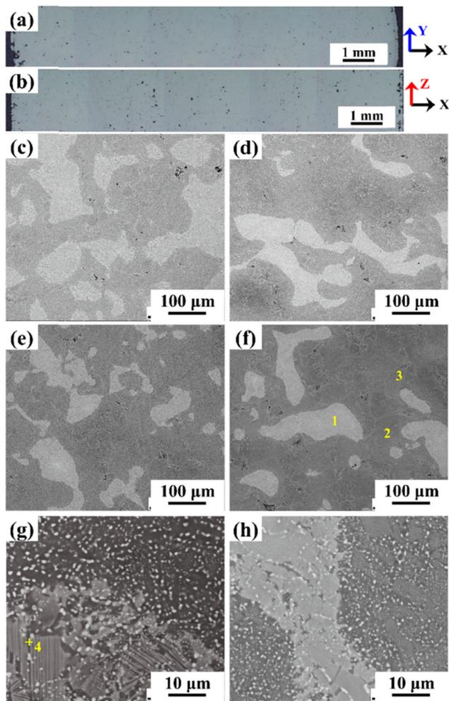
Fig. 7 Microstructure of samples after HIP treatment: optical microscopy images of the (a) 100 W\_M\_HIP\_2 sample along the transverse direction, (b) 100 W\_M\_HIP\_2 sample along the longitudinal direction, and (c) 100 W\_CH\_HIP\_2 sample along the transverse direction. Backscattered electron microscopy images of the samples along the transverse direction: (d) 100 W\_M\_HIP\_2, (e) 80 W\_CH\_HIP\_1, (f) 100 W\_CH\_HIP\_1, (g) 100 W\_M\_HIP\_2, and (h) 100 W\_CH\_HIP\_1.
