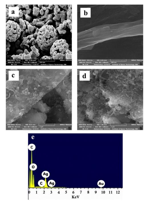
Fig. 4 SEM images of (a) Ag NPs, (b) rGO, (c) Ag@rGO and (d) Ag@rGO/CNT, and (e) EDX graph of Ag@GO/CNT.
