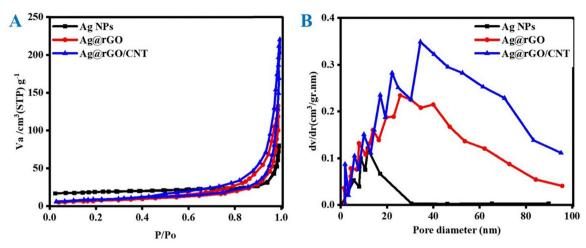
Fig. 5 (A) The isotherm of nitrogen adsorption—desorption and (B) distribution curves of BJH pore sizes for Ag NPs, Ag@rGO, and Ag@rGO/CNT catalvsts.
