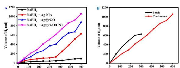
Fig. 6 (A) Time-dependent plot for the hydrolysis of NaBH<sub>4</sub> catalyzed by Ag NPs, Ag@rGO and Ag@rGO/CNT, and in the absence of a catalyst. (B) Comparison of hydrogen development in batch and continuous systems during NaBH₄ hydrolysis.
