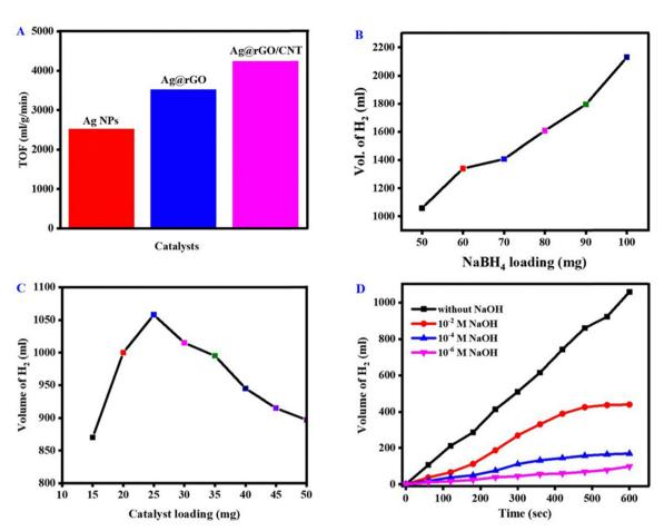
Fig. 7 (A) Turnover frequency in the presence of Ag NPs, Ag@rGO, and Ag@rGO/CNT, (B) effect of NaBH<sub>4</sub> loading, (C) effect of catalyst loading on hydrogen production in the presence of Ag@rGO/CNT, (D) effect of NaOH concentration on hydrogen production in the presence of Ag@rGO/CNT.
