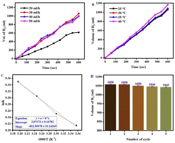
Fig. 8 (A) The impact of the NaBH<sub>4</sub> flow rate on hydrogen production, (B) the relationship between temperature and hydrogen production, (C) Arrhenius diagram generated using the information in Fig. 8, and (D) the stability of the Ag@rGO/CNT catalyst over 4 repetitive cycles.
