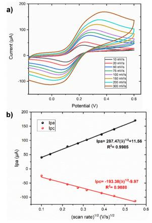
Fig. 7 (a) CV recorded at different scan rates on Cs–MoS $_2$ –SPCEs in 0.1 M KCl containing 5 mM of [Fe(CN) $_6$ ] $^{3-/4-}$ ; (b) plots of the anodic (black) and cathodic (red) peak currents vs. the square root of the scan rate.
