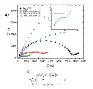
Fig. 8 (a) The Nyquist plots and (b) simulated equivalent circuit of bare and modified SPCEs.
