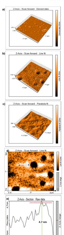
Fig. 2 AFM images of composites deposited on a glass substrate: (a) MoS<sub>2</sub> nanosheets, (b) the Cs-MoS<sub>2</sub> nanocomposite, and (c) chitosan solution, and (d) and (e) the line profile.
