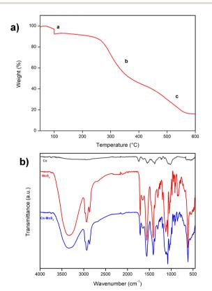
Fig. 3 (a) Thermal stability of the Cs-MoS<sub>2</sub> composite and (b) FTIR spectra of Cs (black line), MoS2 (red line) and the Cs-MoS2 composite (blue line).
