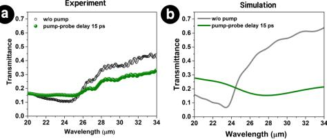
Panel (a) and (b) show the experimental and simulated transmittance of MS1 without a pump and for a pump-probe delay of 15 ps.
