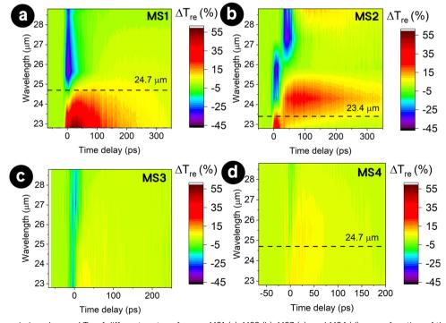
Fig. 6 Transient transmission change  $\Delta T_{\rm re}$  of different metasurfaces – MS1 (a), MS2 (b), MS3 (c), and MS4 (d) – as a function of the pump–probe delay and the FIR wavelength. The horizontal dashed line indicates the plasmonic resonance of the different metasurfaces. The resonance for MS3 (panel c) is not shown because it is out of the range of the figure.
