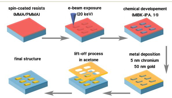
Scheme 1 The schematic representation for the fabrication of plasmonic metasurfaces using the electron beam lithography technique.
