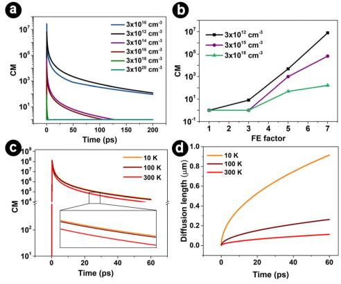
Fig. 1 (a) Time dependence of the carrier multiplication as calculated with the diffusive IMI model. (b) CM at t = 1 ps as a function of the FE factor for different initial carrier concentrations. Panels (c) and (d) show the time evolution of CM and the diffusion length as calculated with the diffusive IMI model at FE = 7 for different sample temperatures.
