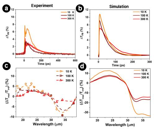
Fig. 3 Measured (a) and simulated (b)  $\Delta T_{\rm re}$  (%) of MS2 as a function of pump-probe delay time for different temperatures (10 K, 100 K, and 300 K) at  $\lambda$  = 22.8  $\mu$ m. Measured (c) and simulated (d) maximal transient change amplitude ( $\Delta T_{\rm max}/T_{\rm t=0}$ ) at different temperatures.
