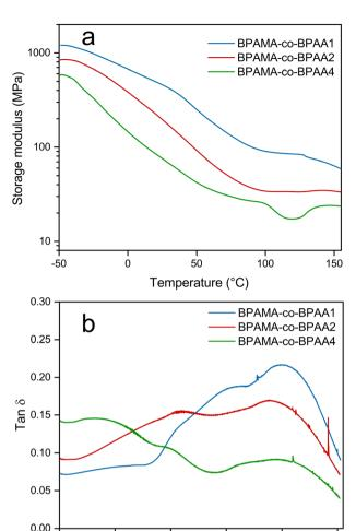
Fig. 6 Storage modulus *versus* temperature (a) and  $\tan \delta$  curve (b) for BPAMA-co-BPAA1, BPAMA-co-BPAA2 and BPAMA-co-BPAA4.
