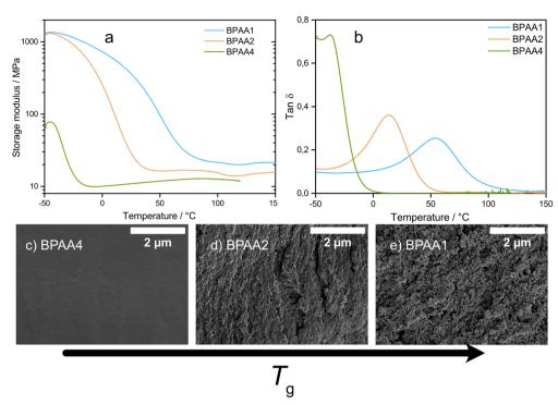
Fig. 5 Storage modulus versus temperature (a) and tan  $\delta$  curve (b) and SEM micrographs of cross sections of (c) **BPAA4**, (d) **BPAA2** and (e) **BPAA4**
