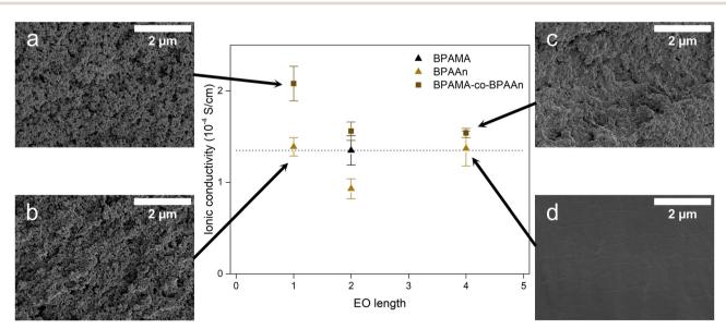
Ionic conductivity for all the samples considered and micrographs referred to (a) BPAMA-co-BPAA1, (b) BPAMA, (c) BPAMA-co-BPAA4 and (d) Fig. 7 BPAA4
