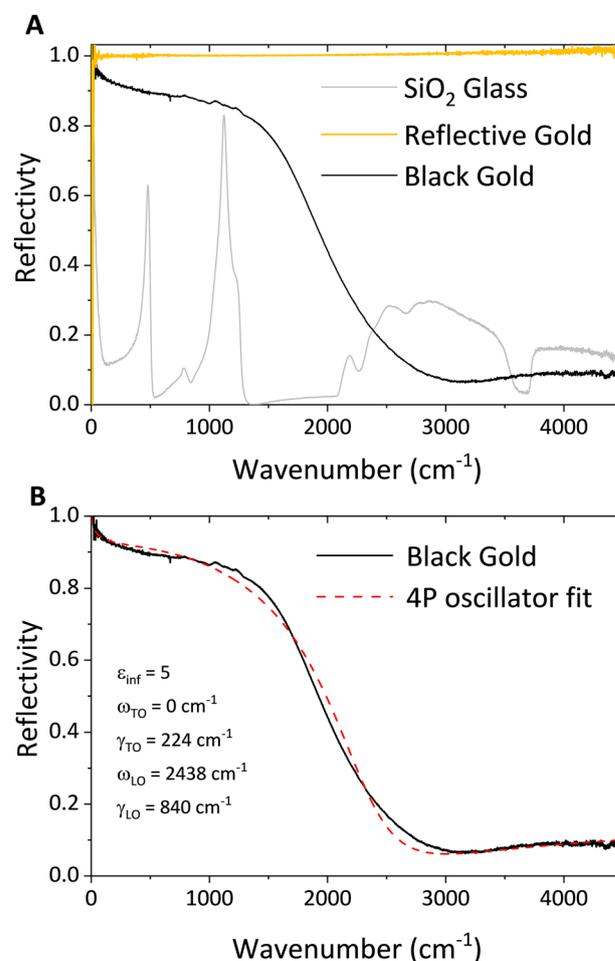
Fig. 9 IR spectra measured in the far and middle infrared regions for the gold films and SiO<sub>2</sub> substrate (A). 4P oscillator fit for the black gold spectrum (B).
