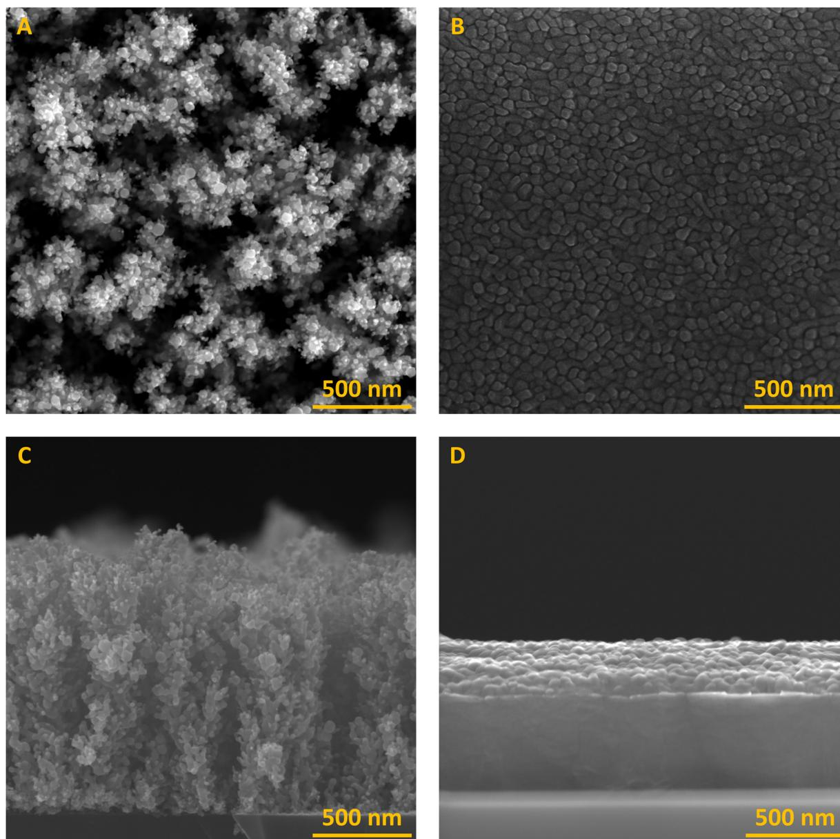
**Fig. 1** Top-down views of the black gold (A) and reflective gold (B) layer taken by applying the electron microscope Tescan MIRA 3, together with the cross-section views of the black gold (C) and reflective gold (D) layers. All the pictures were taken at  $100\,000\times$  magnification and an accelerating voltage of 30 keV.
