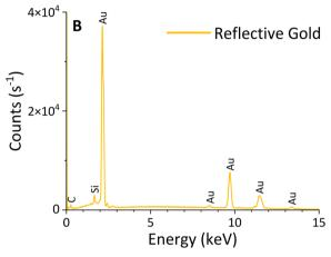
Fig. 2 EDX spectra of black (A) and reflective (B) gold acquired over 5 minutes with an accelerating voltage of 30 keV. A high silicon peak in the BAu spectrum indicates a high porosity of the layer.
