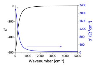
Fig. 10 Real part of the dielectric relative permittivity and optical conductivity of the black gold sample.
