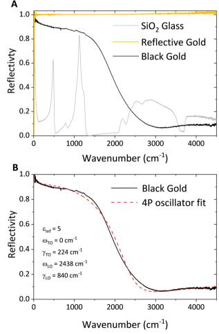
Fig. 9 IR spectra measured in the far and middle infrared regions for the gold films and SiO<sub>2</sub> substrate (A). 4P oscillator fit for the black gold spectrum (B)
