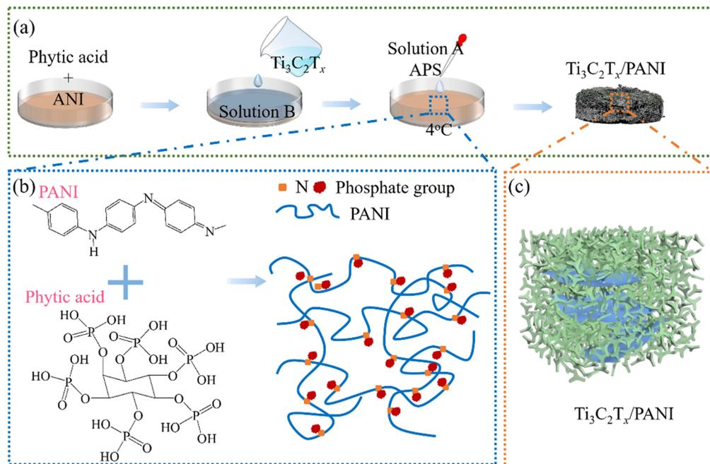
Fig. 1 The synthesis process of porous  $\text{Ti}_3\text{C}_2\text{T}_x/\text{PANI}$  powders. (a) The synthesis process of  $\text{Ti}_3\text{C}_2\text{T}_x/\text{PANI}$ . (b) The crosslinking process of phytic acid and PANI. (c) The structure diagram of  $\text{Ti}_3\text{C}_2\text{T}_x/\text{PANI}$ .
