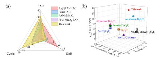
Fig. 6 Comparison of the adsorption performance of  $Ti_3C_2T_x/PANI$  with (a) different PANI related materials and (b)  $Ti_3C_2T_x$  materials (the exact values and references are listed in Tables S2 and S3, ESI.†)
