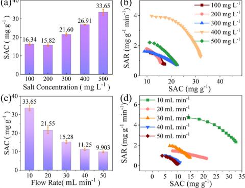
Fig. 5 (a) The plot of salt adsorption concentration and (b) the Ragone curve for Ti<sub>3</sub>C<sub>2</sub>T<sub>x</sub>/PANI at different NaCl concentrations at 1.2 V and 10 mL<sup>-1</sup> min<sup>-1</sup>. (c) The plot of salt adsorption concentration and (d) the Ragone curve for Ti<sub>3</sub>C<sub>2</sub>T<sub>x</sub>/PANI by different flow rates at 500 mg L<sup>-1</sup> NaCl concentration at 1.2 V.
