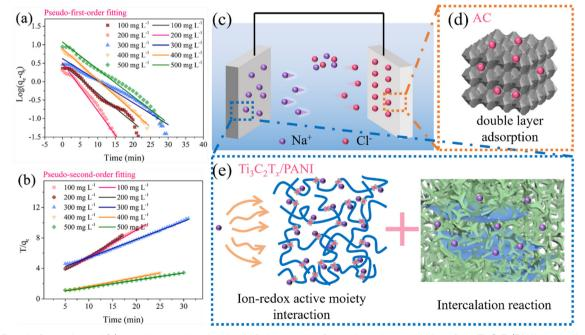
Fig. 7 (a) Pseudo first order and (b) pseudo second order kinetic fitting curves of the adsorption properties of the Ti<sub>2</sub>C<sub>2</sub>T<sub>2</sub>/PANI electrode material at different concentrations. (c) The adsorption process of capacitive deionization for the  $Ti_3C_2T_x/PANI$  electrode. (d) The EDLC ion storage of the AC electrode. (e) The ion intercalation storage process of the Ti<sub>3</sub>C<sub>2</sub>T<sub>x</sub>/PANI electrode.
