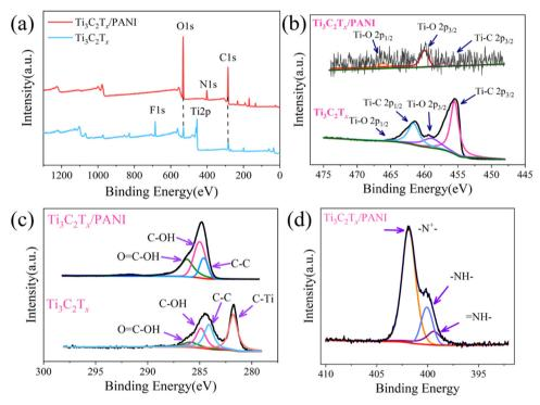
Fig. 4 The XPS spectra of  $Ti_3C_2T_x$  and  $Ti_3C_2T_x/PANI$ . (a) The survey spectra of  $Ti_3C_2T_x/PANI$  and the high resolution XPS spectra of (b)  $Ti_3C_2T_x/PANI$  and  $Ti_$ (c) C 1s and (d) N 1s for  $Ti_3C_2T_x$  and  $Ti_3C_2T_x/PANI$ .
