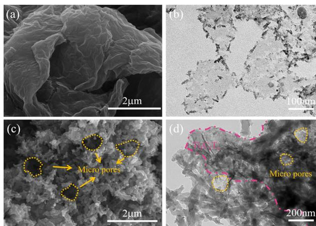
Fig. 2 The SEM and TEM images of different samples. (a) The SEM image of  $\text{Ti}_3\text{C}_2\text{T}_x$ , (b) the TEM image of  $\text{Ti}_3\text{C}_2\text{T}_x$ , and the (c) SEM and (d) TEM images of porous  $\text{Ti}_3\text{C}_2\text{T}_x/\text{PANI}$ .
