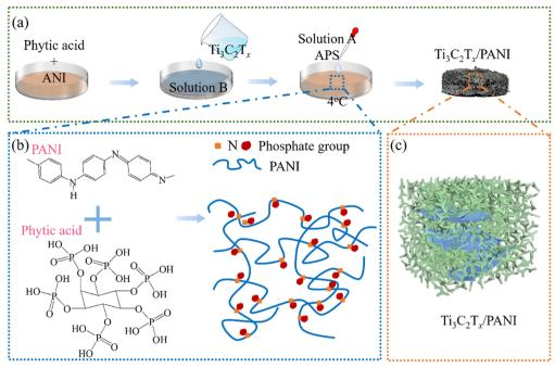
Fig. 1 The synthesis process of porous Ti<sub>3</sub>C<sub>2</sub>T<sub>x</sub>/PANI powders. (a) The synthesis process of Ti<sub>3</sub>C<sub>2</sub>T<sub>x</sub>/PANI. (b) The crosslinking process of phytic acid and PANI. (c) The structure diagram of Ti<sub>3</sub>C<sub>2</sub>T<sub>x</sub>/PANI.
