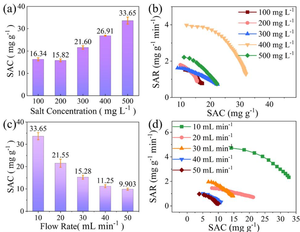
Fig. 5 (a) The plot of salt adsorption concentration and (b) the Ragone curve for  $\text{Ti}_3\text{C}_2\text{T}_x/\text{PANI}$  at different NaCl concentrations at 1.2 V and  $10 \text{ mL min}^{-1}$ . (c) The plot of salt adsorption concentration and (d) the Ragone curve for  $\text{Ti}_3\text{C}_2\text{T}_x/\text{PANI}$  by different flow rates at  $500 \text{ mg L}^{-1}$  NaCl concentration at 1.2 V.
