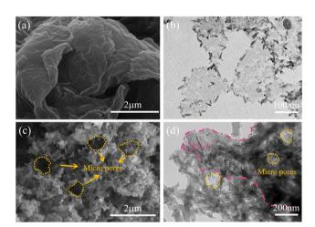
Fig. 2 The SEM and TEM images of different samples. (a) The SEM image of  $Ti_3C_2T_x$ , (b) the TEM image of  $Ti_3C_2T_x$ , and the (c) SEM and (d) TEM images of porous Ti<sub>3</sub>C<sub>2</sub>T<sub>x</sub>/PANI.
