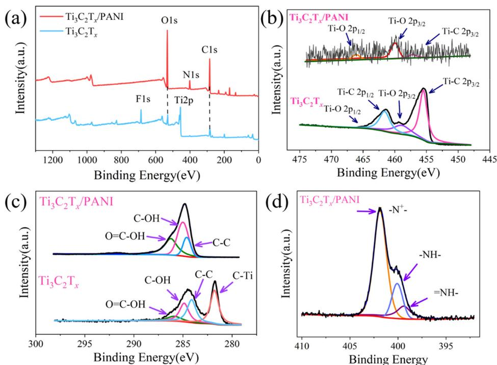
Fig. 4 The XPS spectra of  $\text{Ti}_3\text{C}_2\text{T}_x$  and  $\text{Ti}_3\text{C}_2\text{T}_x/\text{PANI}$ . (a) The survey spectra of  $\text{Ti}_3\text{C}_2\text{T}_x$  and  $\text{Ti}_3\text{C}_2\text{T}_x/\text{PANI}$  and the high resolution XPS spectra of (b) Ti 2p, (c) C 1s and (d) N 1s for  $\text{Ti}_3\text{C}_2\text{T}_x$  and  $\text{Ti}_3\text{C}_2\text{T}_x/\text{PANI}$ .
