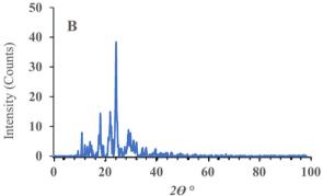
Fig. 4 Powder XRD patterns of plain-SF (A), and SF-NC (B).
