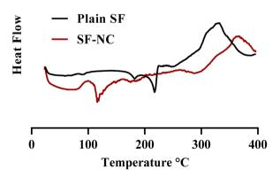
Fig. 3 DSC thermogram of plain SF and SF-NC formulations (F2).
