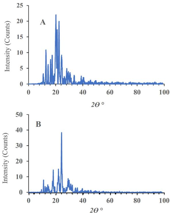
Fig. 4 Powder XRD patterns of plain-SF (A), and SF-NC (B).
