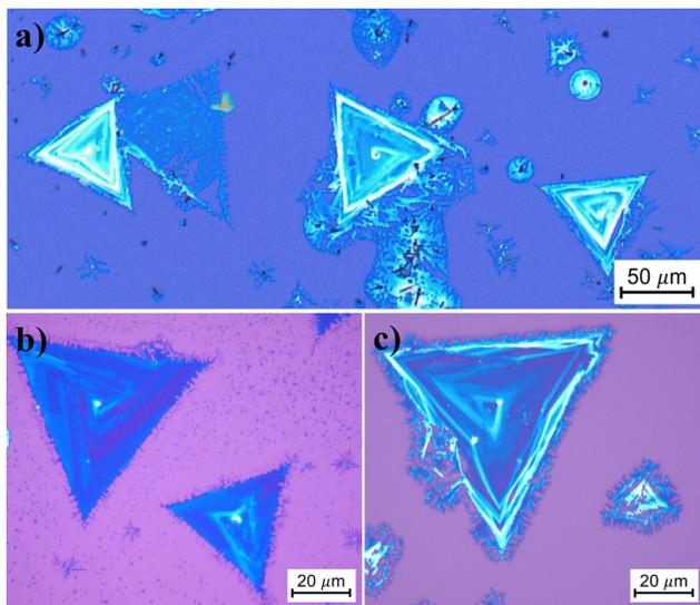
Fig. 11 (a)–(c) High-resolution OM images showing a spiral MoSe<sub>2</sub> pyramid.
