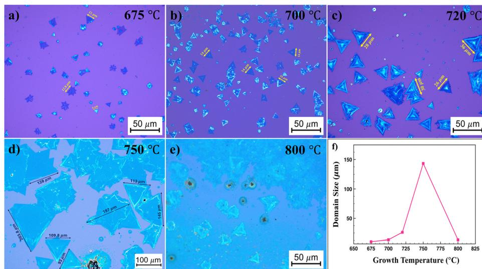
Fig. 6 High-resolution OM images showing variation in the morphology of MoSe<sub>2</sub> on SiO<sub>2</sub>/Si at different growth temperatures using 1.7 mg of NaCl (a)–(e) ranging from 675–800 °C. (f) The domain size of MoSe<sub>2</sub> as a function of growth temperature.
