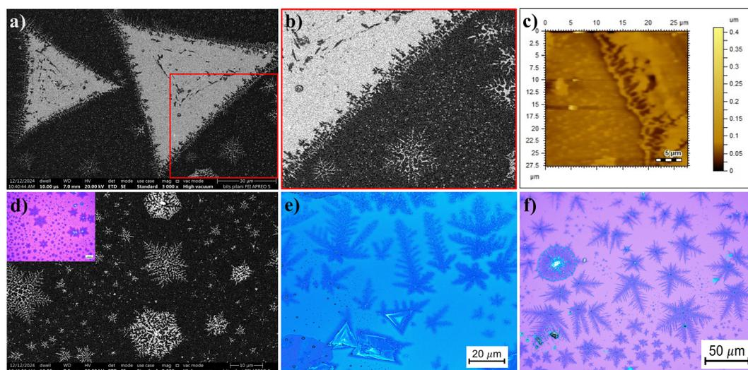
Fig. 10 (a) FESEM image of a  $\text{MoSe}_2$  crystal with fractal edges. (b) Zoomed-in image of the area enclosed in a red square showing the fractals near the edges in Fig. 9(a). (c) AFM image showing the fractal edge of a triangular crystal. (d) FESEM images of snowflakes, inset contains a high-resolution OM image of the same. (e) and (f) High-resolution OM images of the as-grown  $\text{MoSe}_2$  dendrite structures.
