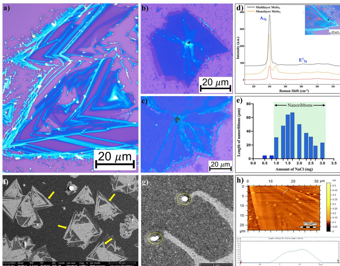
**Fig. 9** (a)–(c) are high-resolution OM images of MoSe<sub>2</sub> nanoribbons. (d) Raman data of the nanoribbons. (e) Plot showing variation in the length of the nanoribbons w.r.t. the amount of NaCl used. FESEM images showing (f) nanoribbons grown along the edges of the MoSe<sub>2</sub> crystals, indicated by yellow arrows; (g) zoomed-in image with an encircled nanoparticle; (h) AFM image and height profile (along the line AB) of the as-grown MoSe<sub>2</sub> nanoribbons.
