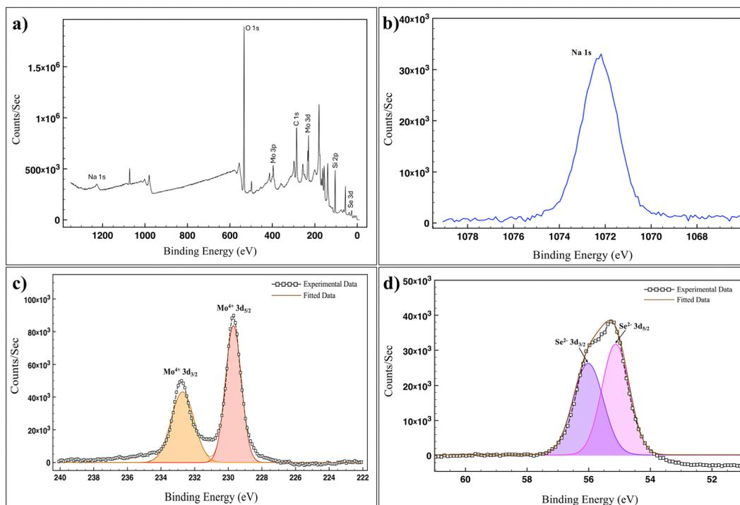
Fig. 5 XPS spectra of MoSe<sub>2</sub> monolayer grown on SiO<sub>2</sub>/Si. (a) XPS survey spectrum. (b–d) Core-level spectra of Na 1s, Mo 3d, and Se 3d, respectively.
