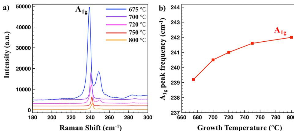
Fig. 7 (a) Temperature-dependent Raman spectra of the MoSe<sub>2</sub> crystal depicting evolution of the Raman peak; different colors represent different temperatures. (b) Frequency peaks of the A<sub>1g</sub> mode plotted w.r.t. growth temperature.
