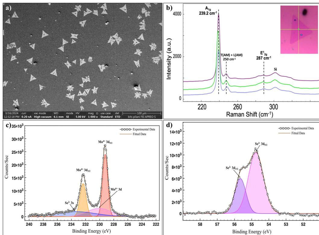
Fig. 2 (a) FESEM image of the as-grown MoSe<sub>2</sub> crystal on the SiO<sub>2</sub>/Si substrate using the standard recipe (without NaCl) at a growth temperature of 750 °C. (b) Raman spectrum of MoSe<sub>2</sub>. High-resolution deconvoluted XPS spectra of (c) Mo 3d and (d) Se 3d.
