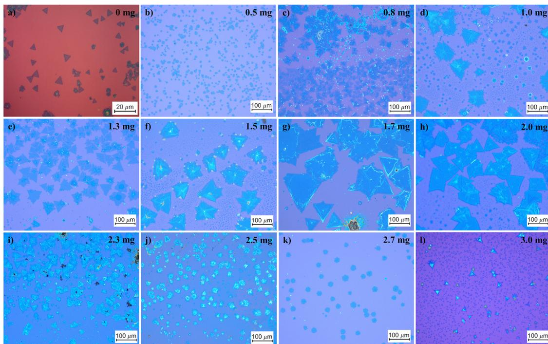
Fig. 3 High-resolution OM images showing variation in the size of the MoSe<sub>2</sub> crystal on the SiO<sub>2</sub>/Si substrate with different amounts of NaCl. (a)–(l) Ranging from 0 to 3 mg at a growth temperature of 750 °C.
