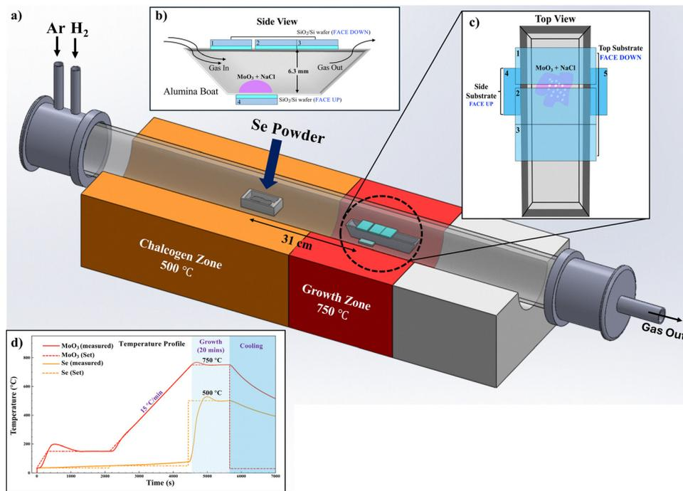
Fig. 1 (a) Schematic illustration showing the experimental set-up for CVD of MoSe<sub>2</sub>; (b) and (c) the side view and the top view of the substrates placed on the alumina boat containing MoO<sub>3</sub> and NaCl, respectively; (d) the temperature profile for the APCVD growth of MoSe<sub>2</sub>.
