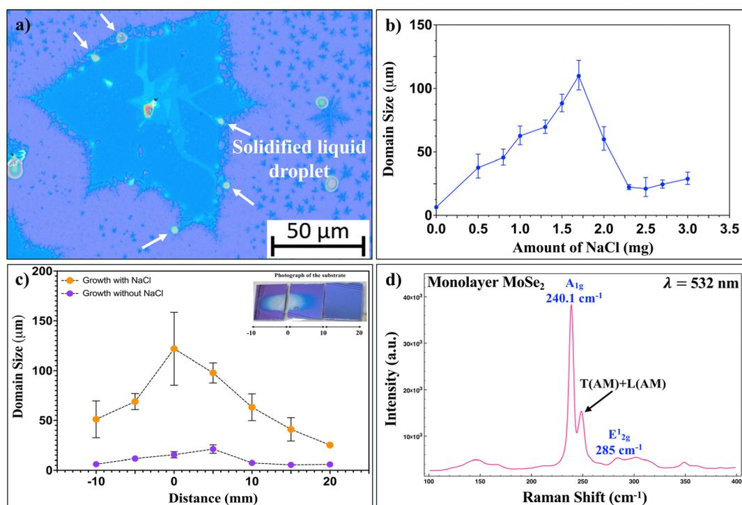
Fig. 4 (a) Optical image of the as-grown MoSe<sub>2</sub> crystal surrounded by solidified liquid droplets. (b) The domain size of MoSe<sub>2</sub> as a function of the amount of NaCl. (c) The domain size of MoSe<sub>2</sub> as a function of the distance between the metal oxide precursor and NaCl precursor to the region of deposition. (d) Raman spectrum of a monolayer MoSe<sub>2</sub> grown using NaCl.
