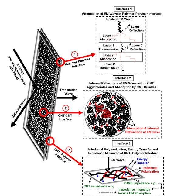
Mechanism of shielding depicting the key events contributing to EMI shielding occurring at the different interfaces
