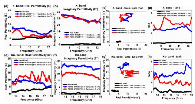
Fig. 8 Dielectric parameters of the test structures: (a) and (b) real and imaginary permittivity of the test structures in the X-band; (e) and (f) real and imaginary permittivity of the test structures in the Ku-band; neat PDMS (black curve), 1 wt% MWCNT sandwiched PDMS (blue curve), and 3 wt% MWCNT sandwiched PDMS (red curve); Cole-Cole plots of the test structures in the (c) X-band and (g) Ku-band;  $\tan \delta$  in the (d) X-band and (h) Ku-band.
