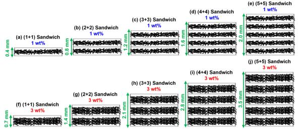
Fig. 4 Schematic of the cross-sectional view of the simulated test structures: (a) – (e) and (f) – (j) are the multilayered stacks in (1 + 1), (2 + 2), (3 + 3), (4 + 4), and (5 + 5) designs based on the experimentally fabricated test structures at 1 wt% and 3 wt% MWCNT concentration on PDMS, respectively. The image is not to scale and is only for representative purposes.
