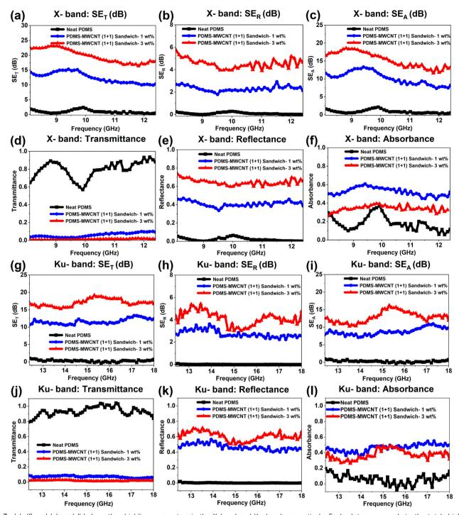
Fig. 7 (a)–(f) and (g), and (h) show the shielding parameters in the X-band and Ku-band, respectively. Each plot corresponds to the total shielding effectiveness ( $SE_7$ ) ((a) and (g)), shielding effectiveness due to reflection ( $SE_R$ ) ((b) and (h)), and shielding effectiveness due to absorption ( $SE_A$ ) ((c) and (i)). The power coefficients governing the shielding effectiveness are also shown individually for (d) and (j) transmittance, (e) and (k) reflectance and (f) and (l) absorption.
