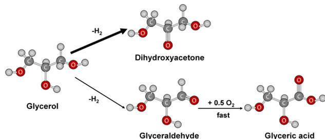
Fig. 5 Reaction scheme of partial glycerol oxidation.
