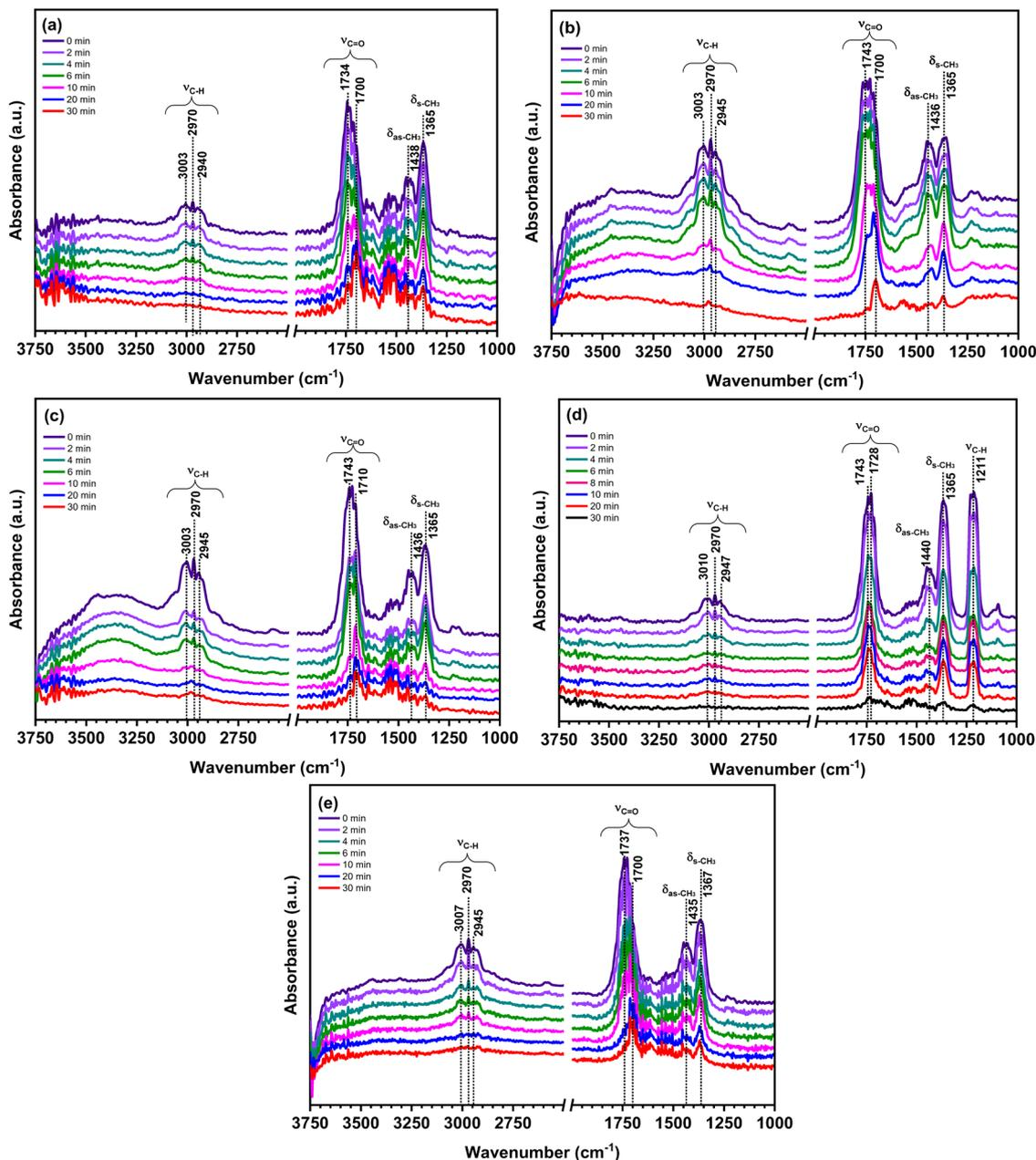
Fig. 8 *In situ* DRIFT spectra of acetone adsorption followed by desorption at 0, 5, 10, 20 and 30 min at 80 °C (from top to bottom) on (a) DM400 (Cu–Co 5%) 400, (b) DM600 (Cu–Co 5%) 600, (c) DM800 (Cu–Co 5%) 800, (d)  $\text{CuCo}_2\text{O}_4$  and (e) DM400.
