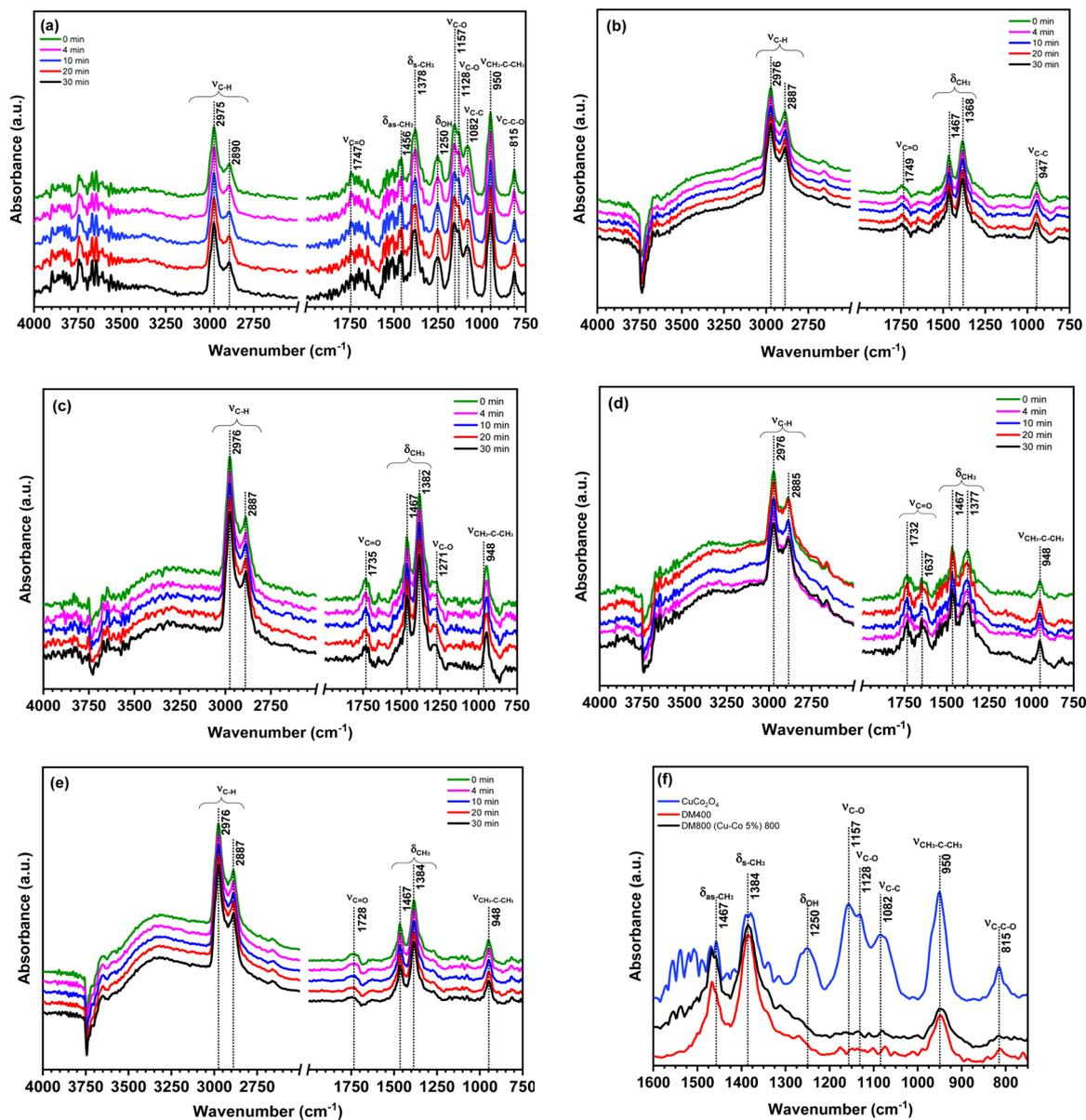
Fig. 6 *In situ* DRIFT spectra of IPA adsorption followed by desorption at 0, 5, 10, 20 and 30 min (from top to bottom) on (a)  $\text{CuCo}_2\text{O}_4$  (b) DM (c) DM400 (Cu–Co 5%) 400, (d) DM600 (Cu–Co 5%) 600, (e) DM800 (Cu–Co 5%) 800 and (f) comparison between DM400, DM800 (Cu–Co 5%) 800 and  $\text{CuCo}_2\text{O}_4$ .
